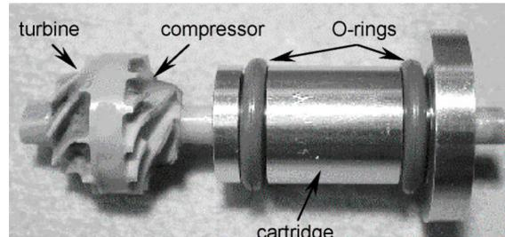
Fig1. Silicon Nitride Turbine compressor group
