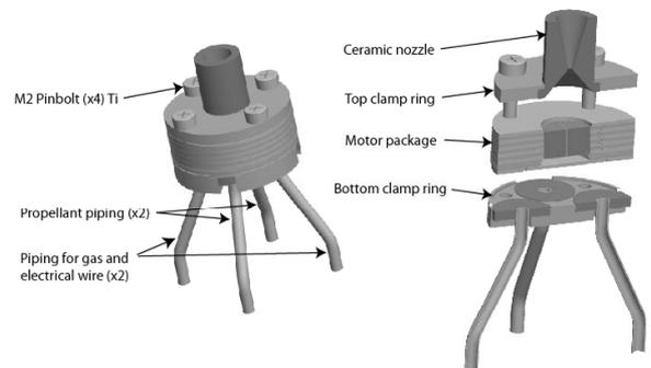
Figure 3: Identification of the key components of the updated DDM concept
