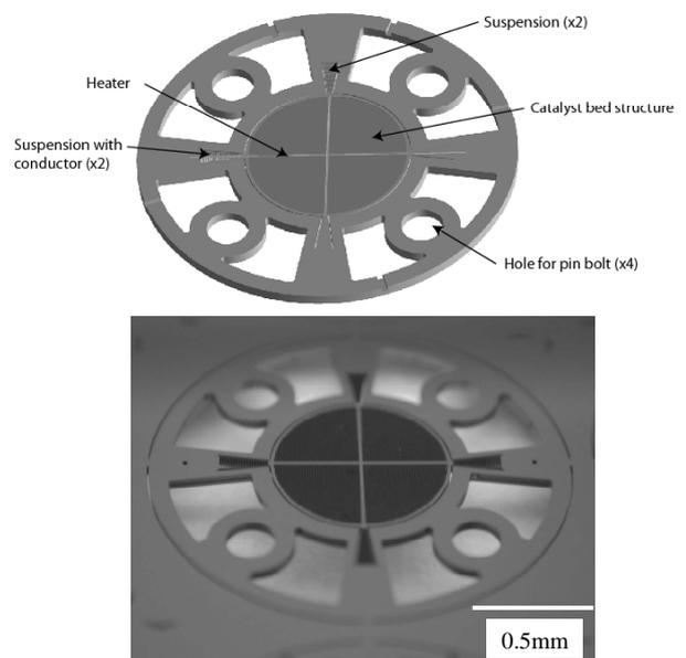
Figure 2: (Top) Layout of a single catalyst bed wafer. (Bottom) A sample catalyst bed wafer from an early fabrication trial
