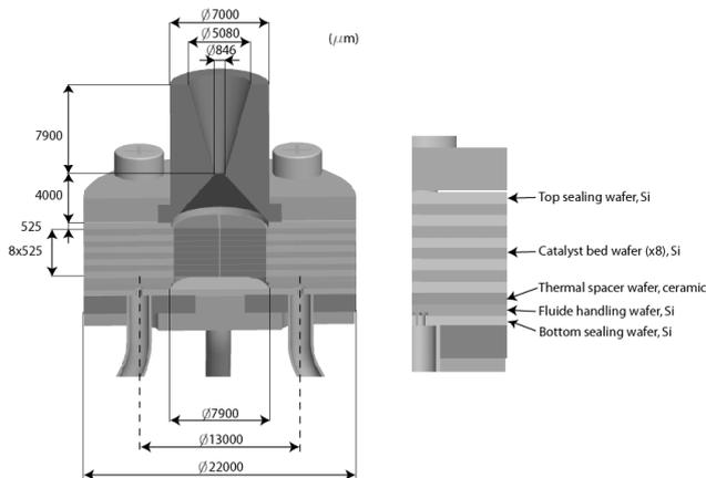
Figure 4: Basic geometry of the motor assembly in the monopropellant concept
