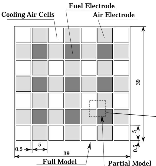
does not exist) there would be certain amount of heat transfer between elements in the actual model. Therefore, expected more moderate temperature distribution than the result of this calculation.
