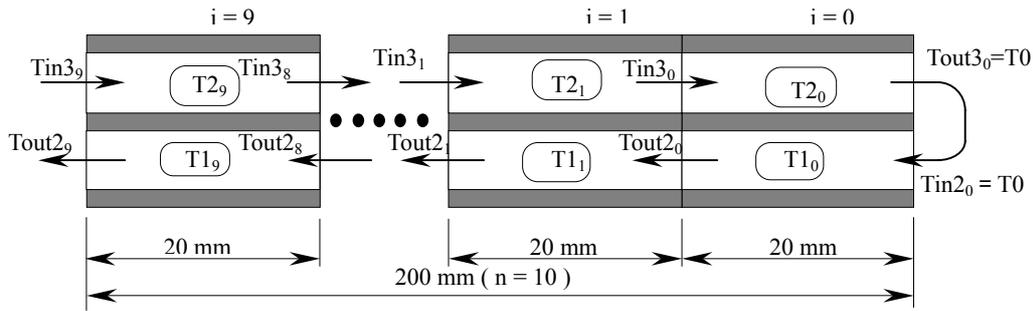
**FIG.6 Typical Temperature Distribution of Honeycomb Type Regenerative SOFC**
