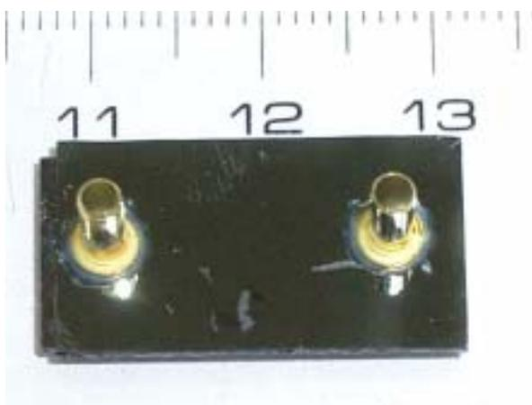
Figure 4. Macroporous micro channel reactor with a ruthenium catalyst supported into a macroporous silicon structure.
