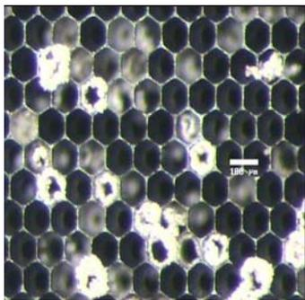
Figure 6: Granular deposits at the pipe orifices. These are normally removed using a pumped electroless plating setup.
