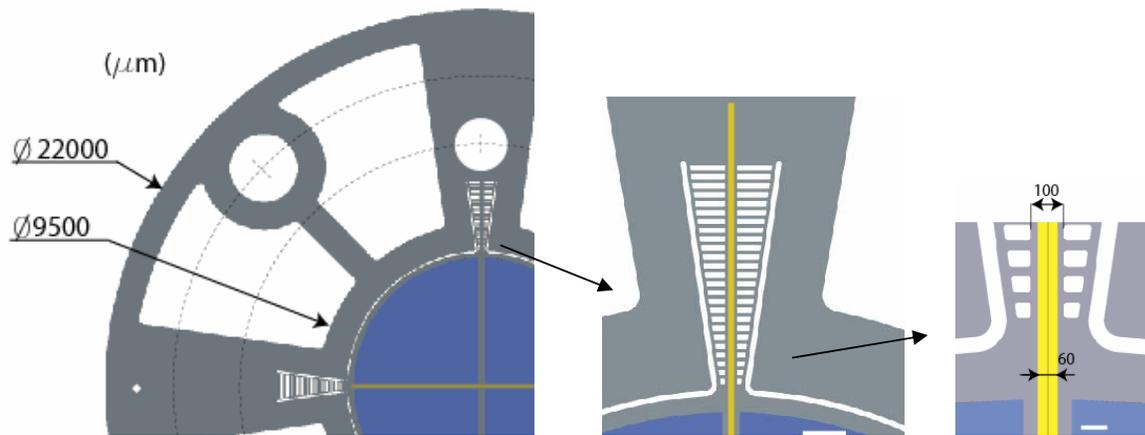
Figure 3: Detailed design of the catalyst wafer. All dimensions are in micrometers. Each wafer is 525 micrometers thick. From left to right: 1. The overall dimensions of the catalyst bed. 2. The details of a suspension strut containing a heater path. One pair of struts has this feature, whilst the other pair has not. 3. Fine details of the strut interface to the catalyst bed structure.
