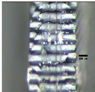
Figure 7: Cross-sections of the catalyst bed structure, showing the conformal silver coating achieved by non-pumped electroless plating. The cross section is made by cleaving, which leaves a very rough section. The bright, reflecting surfaces are silver.
