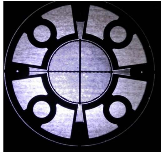
Figure 4 – A top picture of the catalyst bed wafer which is illuminated from below. It can be seen that the vertical suspending beams, in difference to the horizontal, lack heater conductor beams. Outside the horizontal suspending beams the electrical via holes can be seen.
