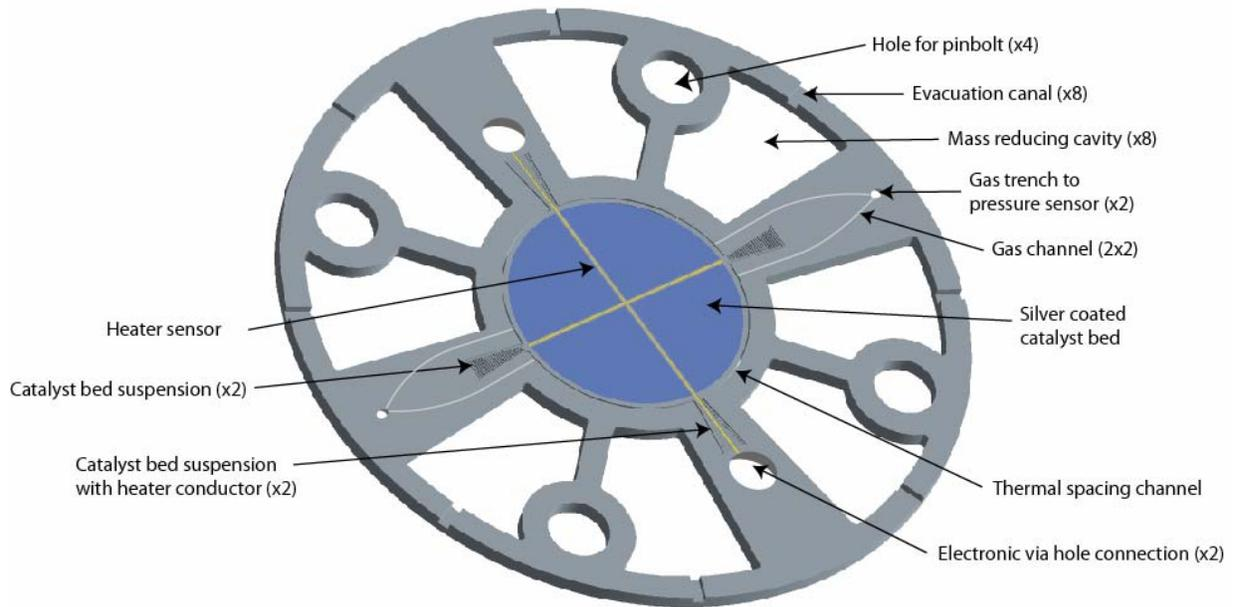
Figure 2: Catalyst wafer overview. All different functional parts are indicated. Eight similar small wafers are laminated in order to form a catalyst pack. The darker circular area in the middle contains the honeycomb structure, carrier of the catalyst coating. The honeycomb structure is suspended by four struts from the surrounding bulk silicon structure, enabling reduced thermal conductance from the device.
