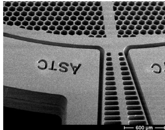
Figure 5 – A SEM picture of the honeycomb suspending beam. The conductor pattern is clearly visible, but not metallized. The thermal spacing surrounding the honeycomb structure is 50µm wide.
