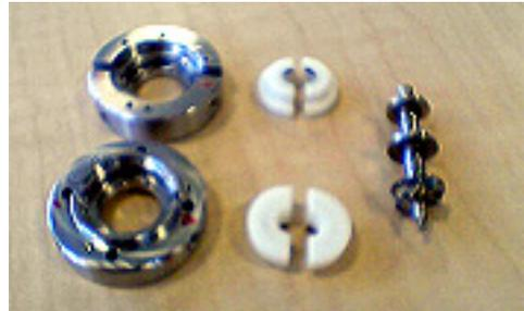
Figure 13. Photo of the shaft and the bearings
