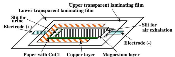
Fig. 1. Schematic diagram of a urine-activated paper battery: a Copper (Cu) film, Copper Chloride (CuCl)-doped filter paper, and a Magnesium (Mg) film are stacked and laminated between two transparent laminating films. Two slits are made to contact urine to the paper and remove the air from the battery.
