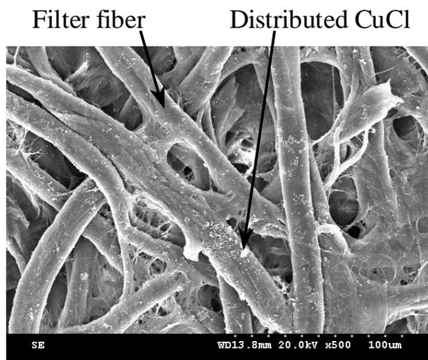
Fig.4. SEM photograph of the paper with CuCl: CuCl is distributed on the filter paper fiber.
