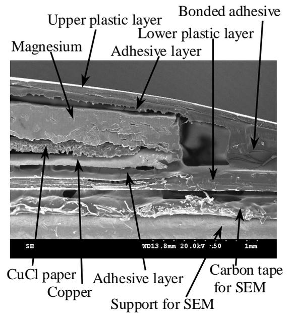
Fig.7. SEM micrograph of the cross-section of the laminated battery: the CuCl-doped paper contacts both Magnesium (Mg) and Copper (Cu). Adhesive of the upper and lower plastic layers adhered all layers together after heating.
