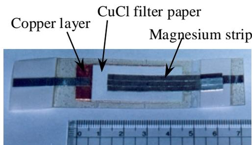
Fig.6. Photograph of the prototype paper battery: the size is 6cm x 3cm.
