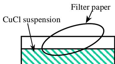
(a) Soaking filter paper in CuCl suspension
