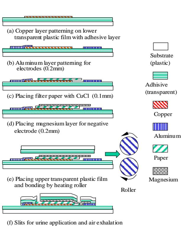
Fig.5. Fabrication process for the paper battery: the stacked layers of the Copper (Cu), CuCl-doped filter paper, and Magnesium (Mg) between the two transparent plastic films are laminated while passing through heating rollers. Adhesive on the plastic film bonds all material together by the heat and pressure of the rollers.
