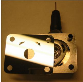
**Figure 4.** The UC Berkeley Wankel engine next to a silicon wear plate.
