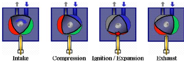
Figure 2. The four steps in the Wankel engine cycle.
