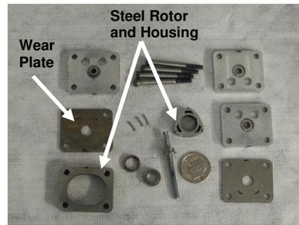
Figure 3. The parts for a micro Wankel engine compared to the size of a US dime. The wear plate shown will be outfitted with a MEMS sensor network.
