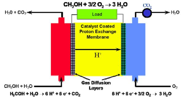
**Figure 5.** Schematic for a direct methanol fuel cell.
