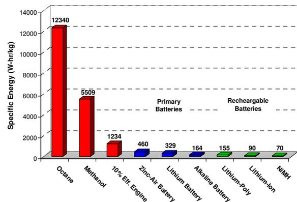
**Figure 1. A comparison of the specific energy of common fuels with both rechargeable and primary batteries.**
