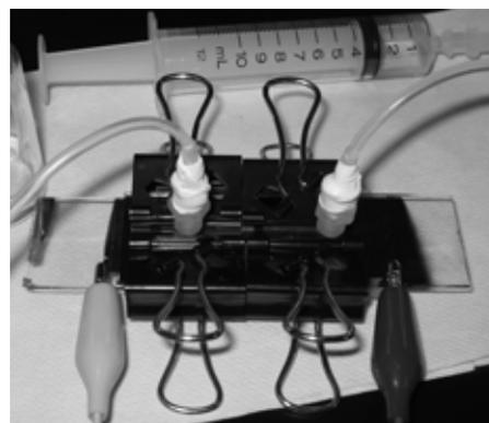
Figure 3. The illustration (upper) and photograph (lower) of the construction of the microfluidic fuel cell to evaluate the performance of enzyme electrode under the steady fuel flow.
