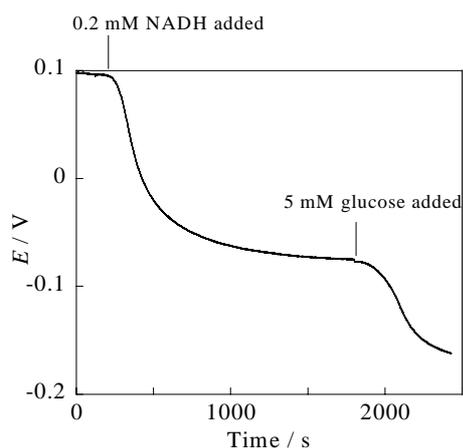
Figure 8. Time courses of the rest potential of PAA-VK3-Dp electrode, which is placed below the GOD membrane. 5 mM glucose followed by the addition of 0.2 mM NADH was added (pH 7, air saturated).
