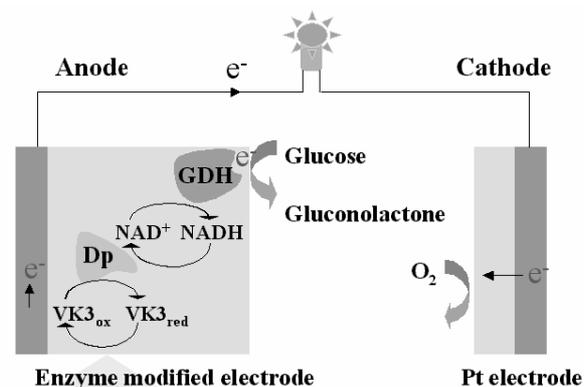
Figure 1. Schematic illustration showing the construction of Dp / GDH biofuel cell and the principle for generating electricity from biofuel (glucose in this case).
