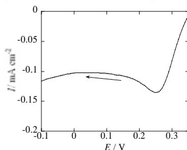
Figure 5. A linear sweep voltammogram for a PDMS-coated Pt plate in air-saturated PBS at 5 mV / s.
