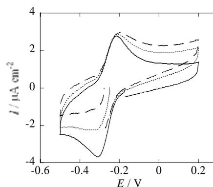
Figure 6. Cyclic voltammograms of the electrode coated with PAA-VK3 - Dp - GDH at 50 mV / s. Buffer only (solid line); 0.5mM NADH (dotted line); 0.5 mM NADH and 10 mM glucose (broken line)
