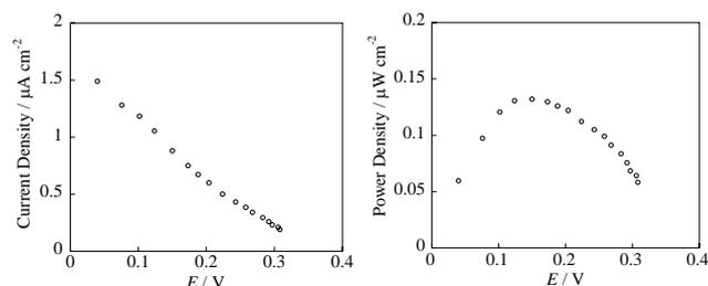
Figure 7. Dependence of the current density (left) and the power density (right) on the voltage of the biofuel cell (pH 7.0, at 25 °C). Fuel is air-saturated PBS containing 5mM glucose and 1 mM NADH.
