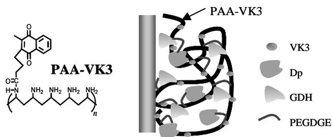
Figure 2. The molecular structure of PAA-VK3, and an illustrated structure of the composite film of Dp, GDH and PAA-VK3 cross-linked by PEGDGE.
