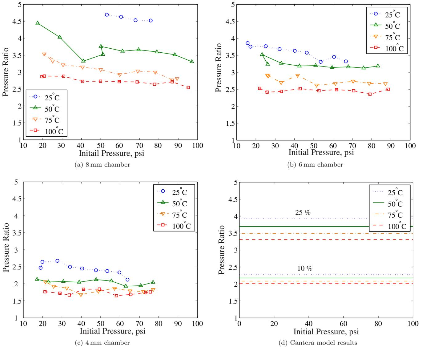
Figure 5. Pressure ratio against the initial pressure.
