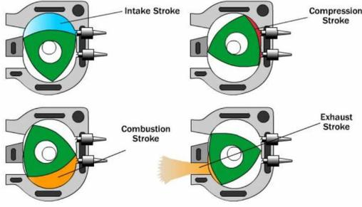
Figure 1. Four-stroke cycle of Wankel engine.
