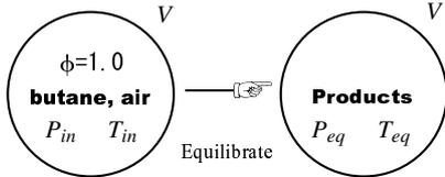
Figure 4. Schematic of constant volume combustion bomb model.
