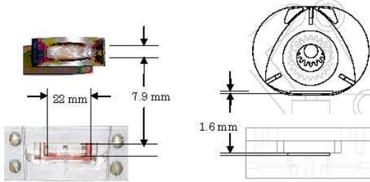
Figure 2. Dimensions of a Wankel engine combustion chamber.
