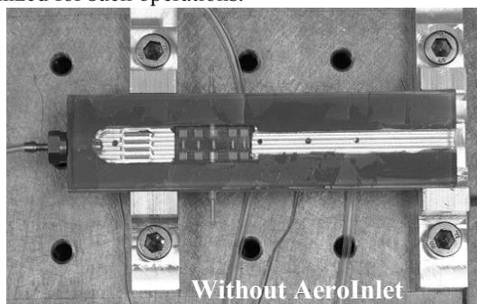
Figure 3. The spark electrode and evaporator chip in a  $\sim 3x$  scale combustor for single shot tests. The combustor tail section is 5cm long.
