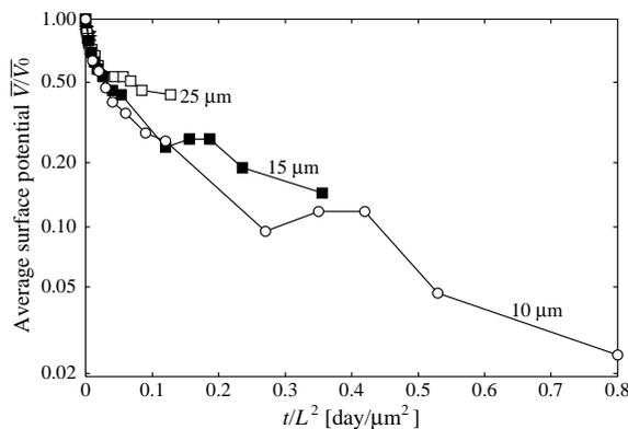
Figure 12: Surface potential decay of micropatterned electrets treated by fluorinated silane coupling agents (normalized time scale)
