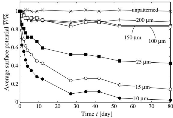
Figure 10: Surface potential decay of micropatterned electrets treated by fluorinated silane coupling agents (real time scale)
