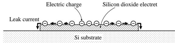
Figure 9: Charge disappearance by leak current through the surface
