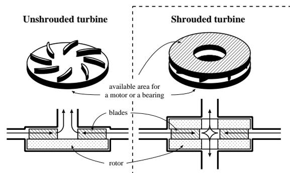
Figure 2: Schematic structure of a shrouded turbine
