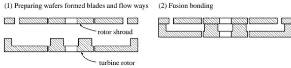
Figure 3: Fabrication process of a shrouded turbine without using cavity through etching
