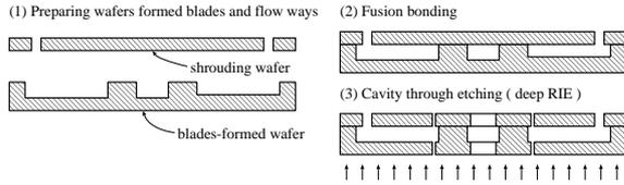
Figure 4: Fabrication process of a shrouded turbine with using cavity through etching
