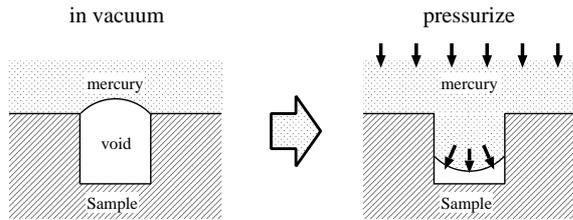
Figure 8: Pressurizing process to improve contact with mercury
