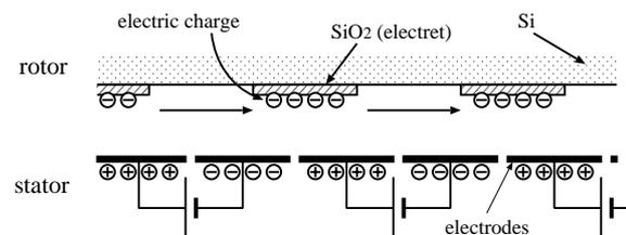
Figure 1: Schematic cross section of the electret motor
