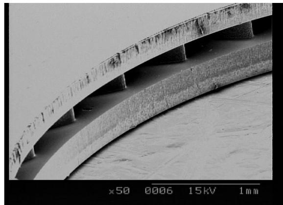
Figure 6: SEM photograph of a stator
