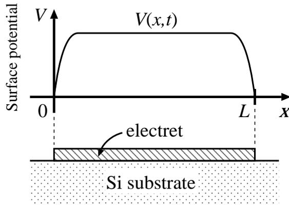
Figure 11: The electret model in the surface decay analysis
