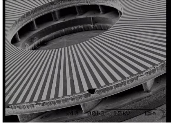
Figure 5: SEM photograph of a shrouded turbine
