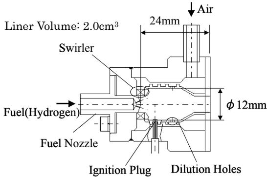
Fig 8. Cross section of the 2cc micro-combustor for Hydrogen fuel
