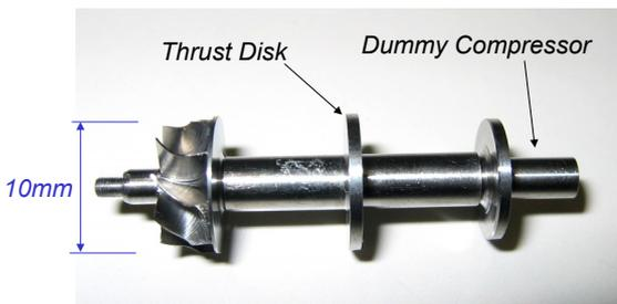
Figure 3. Rotor used for the micro-bearing test
