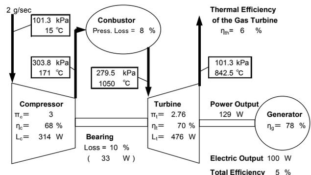
Fig.1 Target cycle of the 100W class micro-scale GT
