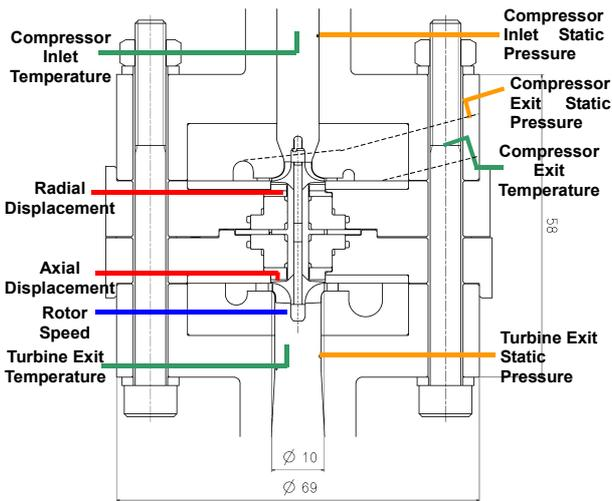
Figure 5. Cross section and the instrumentation of the micro-compressor test rig
