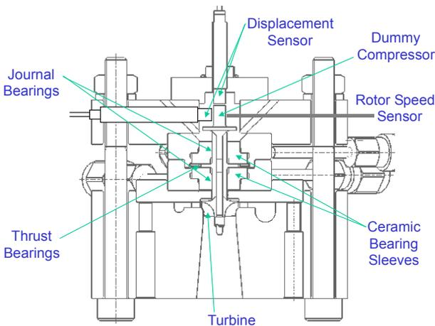
Figure 2. Cross section of the micro-bearing tester
