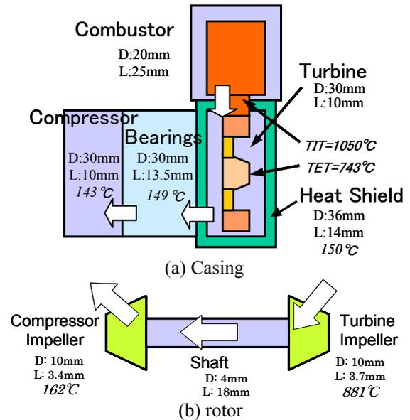
Fig 10. Heat conduction calculation results
