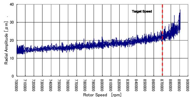
Fig.4 Radial amplitude of the rotor vibration
