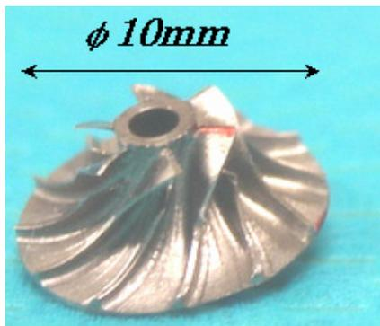
Fig 6. Close-up view of the micro-compressor impeller
