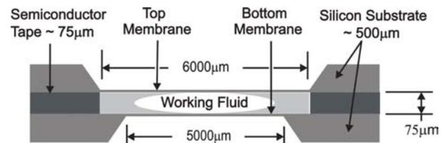
Figure 1. Engine Cross-Section
