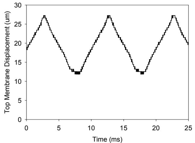
Figure 7. 100Hz Operation using Thermal Switch Heat Rejection
