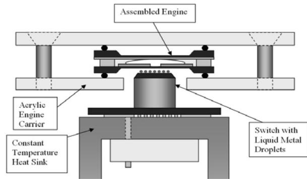
Figure 2. Engine and Thermal Switch
