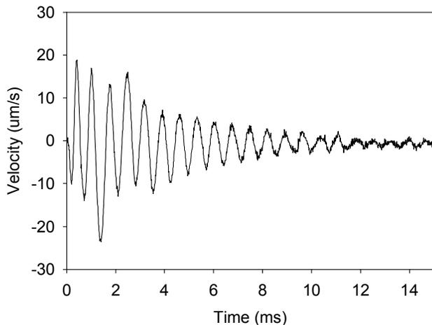
Figure 3. Top Membrane Ringout
