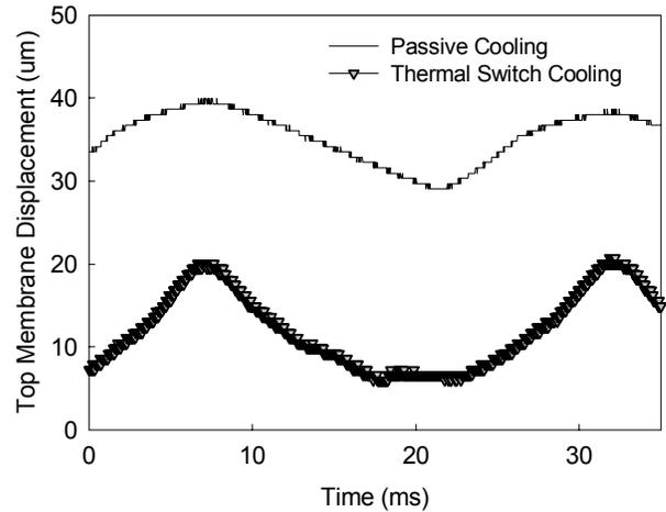
Figure 5. Heat Rejection via Thermal Switch
