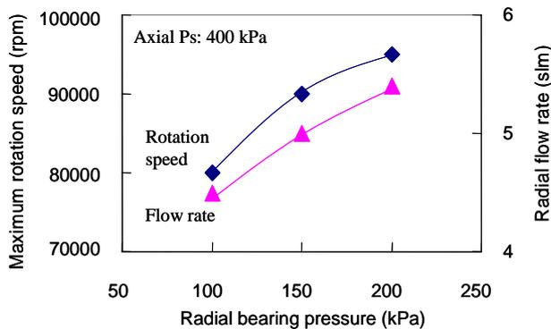
Fig. 10. Maximum rotation speed at different radial bearing pressures
