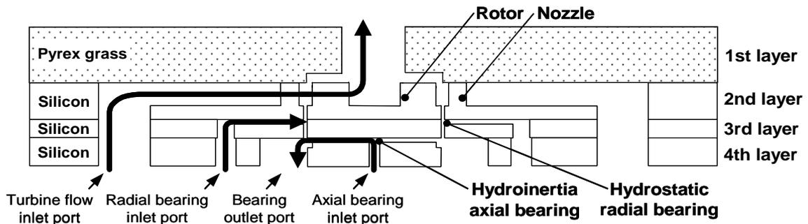
Fig. 1. Cross sectional structure of the air turbine
