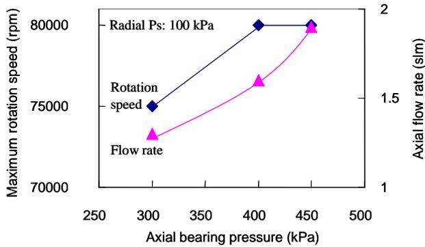
Fig. 9. Maximum rotation speed at different axial bearing pressures
