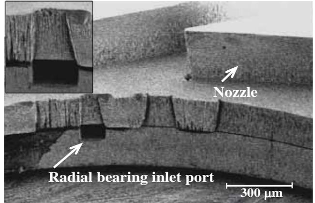
Fig. 7. Rough radial bearing housing fabricated by cavity-through DRIE
