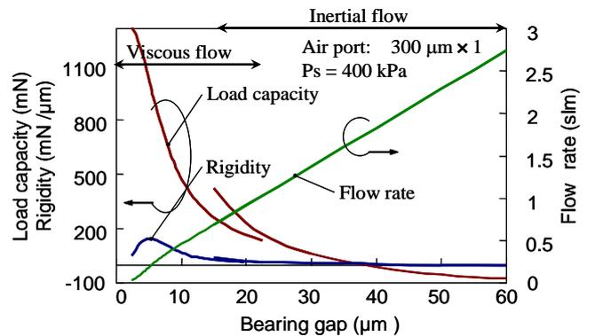
Fig. 5. Design calculation of the hydroinertia axial bearing
