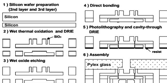
Fig. 6. Fabrication process
