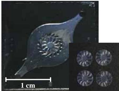
Fig. 2. Fabricated rotors and stator
