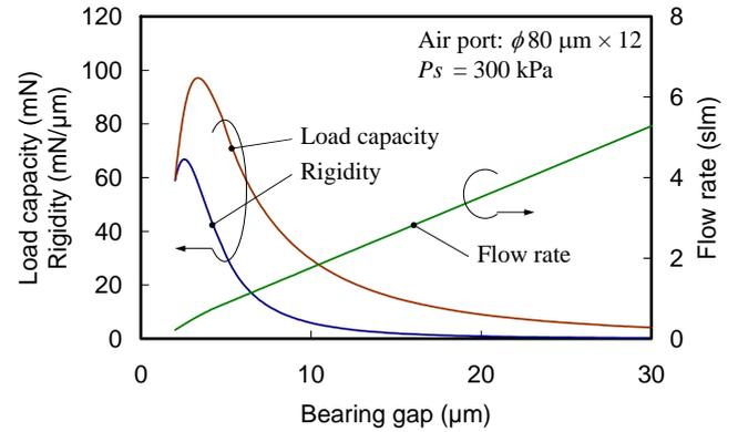
Fig. 4. Design calculation of the hydrostatic radial bearing
