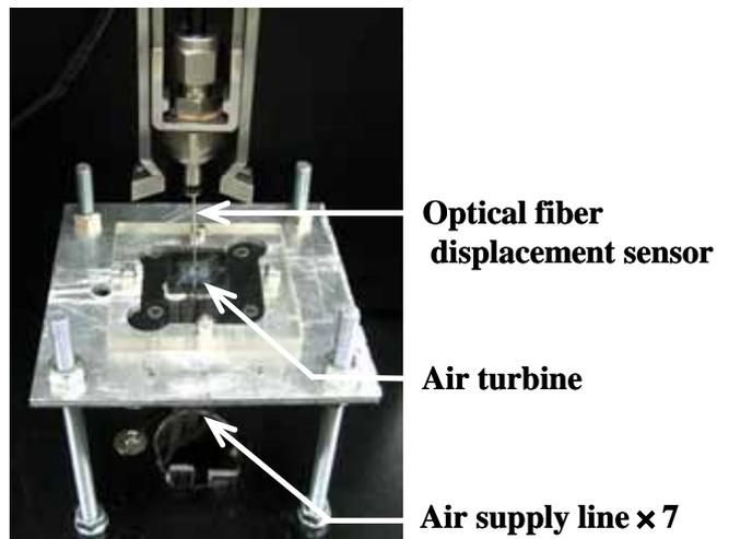
Fig. 8. Setup for the MEMS-based turbine
