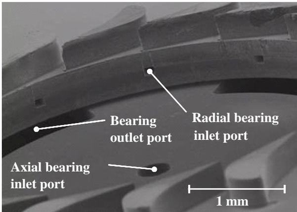
Fig. 3. Gas lubrication system
