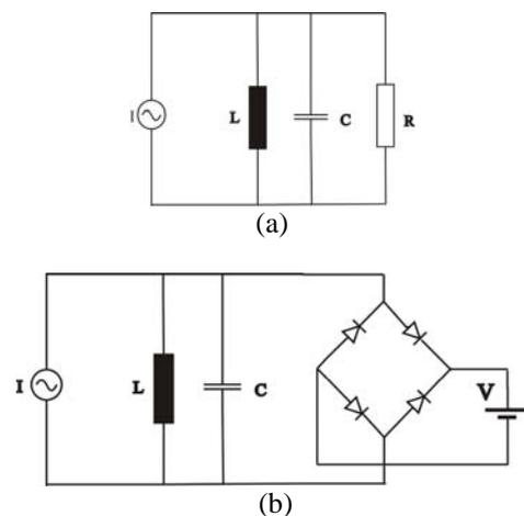
Figure 1. Basic resonance structure with (a) linear load and (b) non-linear load.
