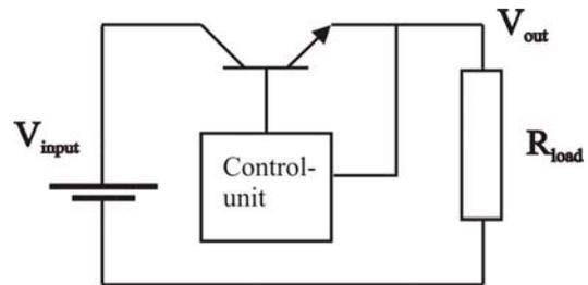
Figure 4. Series linear voltage regulator
