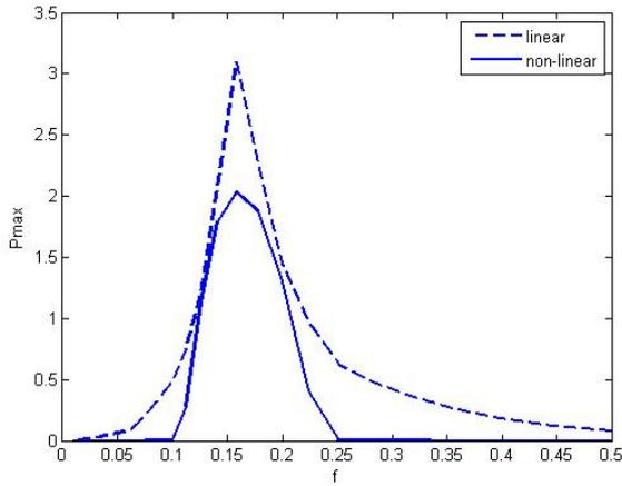
Figure 2. Maximum load-voltage versus frequency of the resonance structure.
