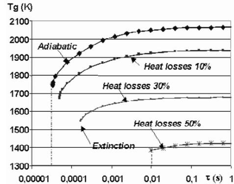
Figure 4 : Gas temperature versus residence time for different levels of heat losses (CH<sub>4</sub>)
