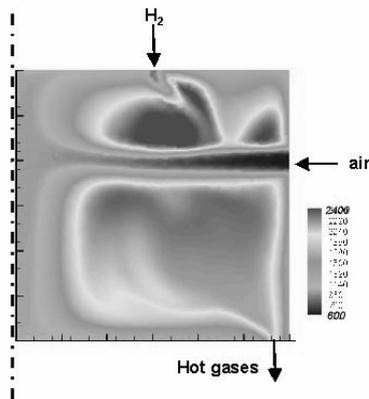
Figure 6 : computed temperature field
