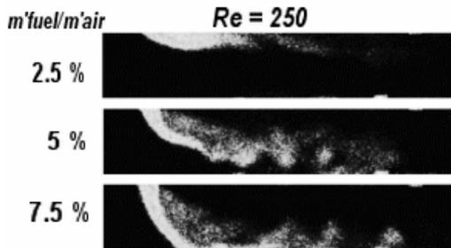
Figure 3 : Images three mass flow rates (Re = 250)
