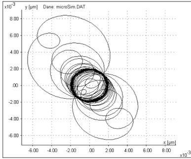
Figure 9 Nonlinear orbit calculation for 1 million rpm micro gas bearing
