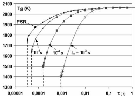
Figure 5 : Gas temperature versus residence time for different mixing time scales ( $CH_4$  without heat loss)
