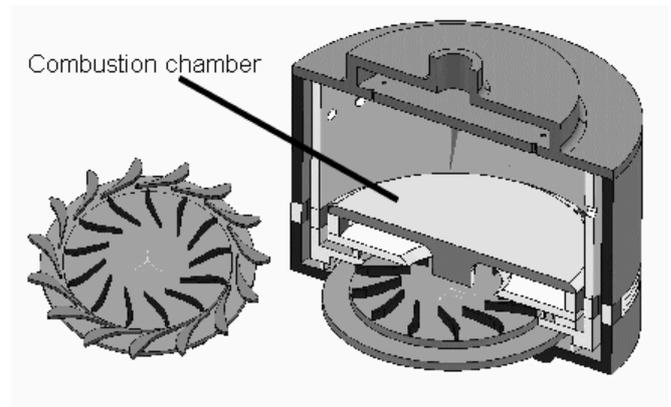
Figure 1 : proposed microturbine concept
