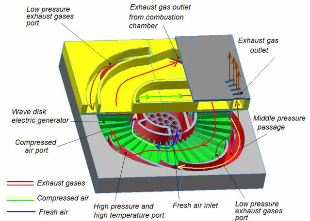
Fig. 2 Details of the one step compression wave engine construction
