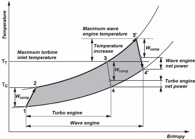
Fig.1 Schematic Temperature-Entropy diagram for turbo-engine and wave-engine.
