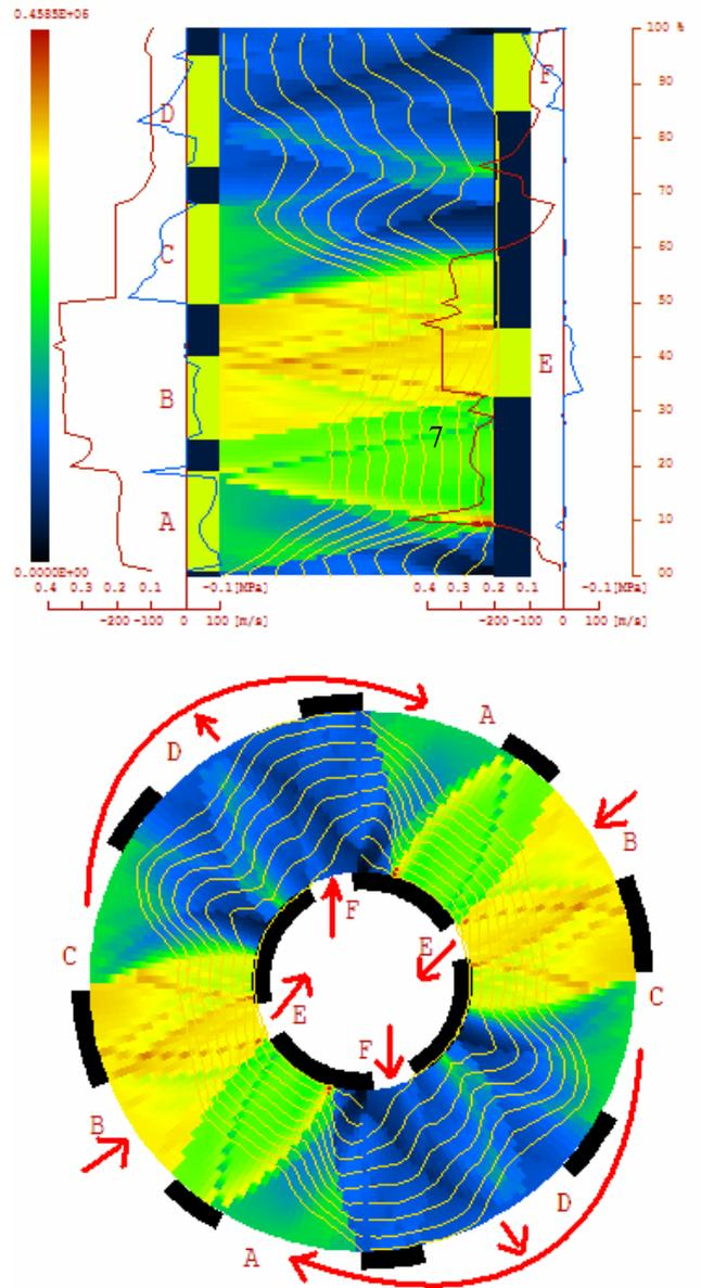
Fig. 4 Pressure distribution inside the wave disc of the two step compression wave engine.
