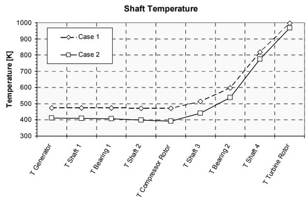
Figure 8. Simulated temperature distribution in the shaft for two slightly different machine layouts.
