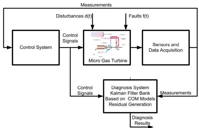
Figure 6. Model-based and control-oriented diagnosis of the micro gas turbine.
