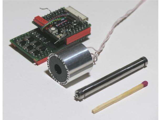
Figure 7. Rotor including two permanent-magnets and assembled high-speed ball bearings, stator with three phase winding, power and control electronics.
