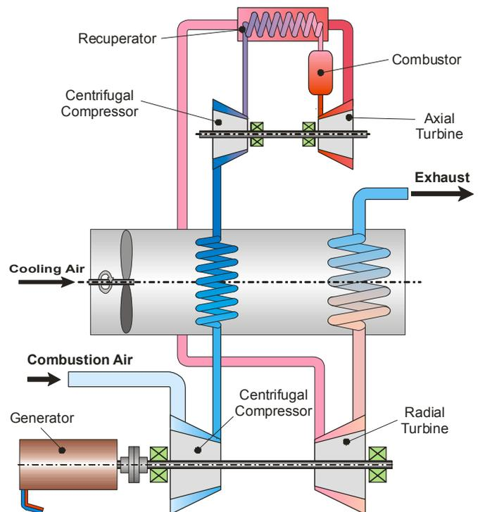
Figure 2. Setup of a two-stage gas turbine system.
