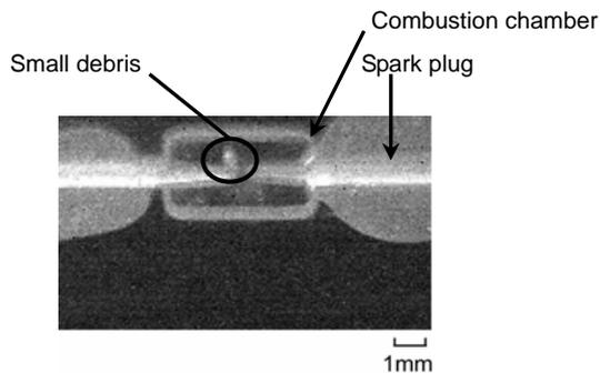
Figure 8. Si debris due to wear
