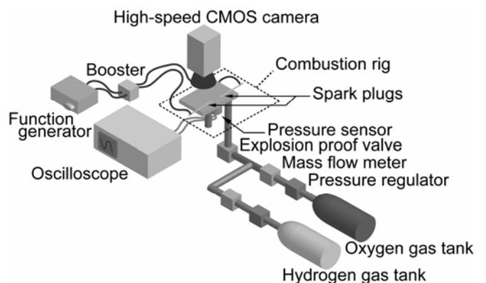
Figure 4. Schematic of experimental instruments
