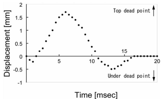
Figure 7. Displacement of piston
