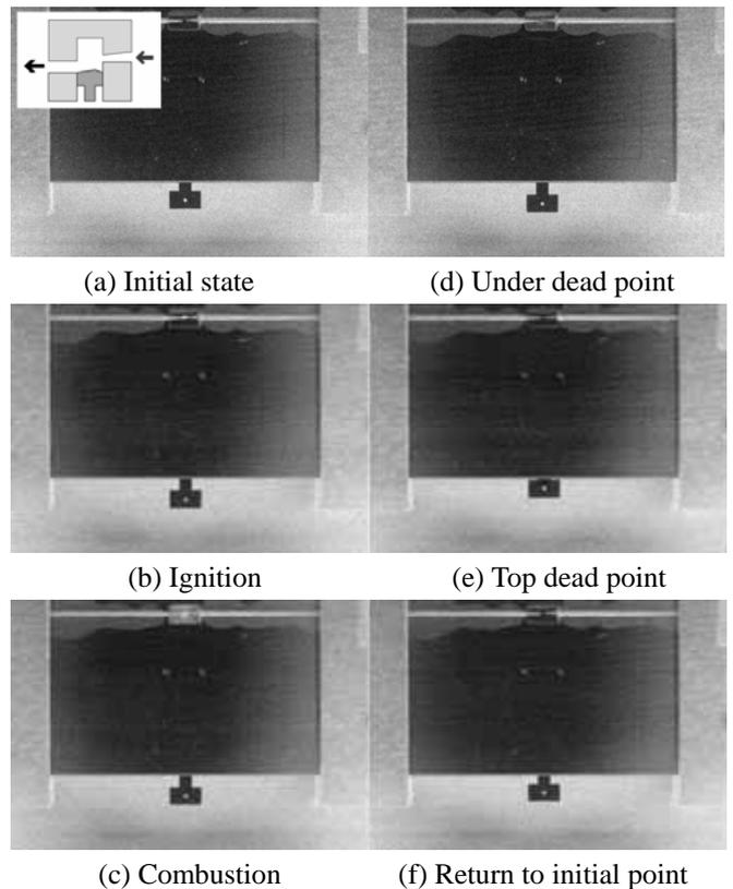
Figure 6. High-speed CMOS camera images of the piston motion
