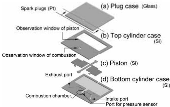
Figure 1. Structure of the combustion rig
