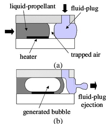
Figure 1. Working principle of the microthruster using low boiling temperature liquid-propellant with high-viscous fluid-plug; (a) the propellant and plug before ejection; (b) the propellant and plug at ejection.
