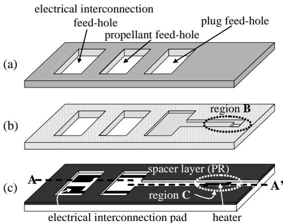
Figure 3. Perspective view of the microthruster layers: (a) top polymer layer; (b) middle silicon layer; (c) bottom glass layer.
