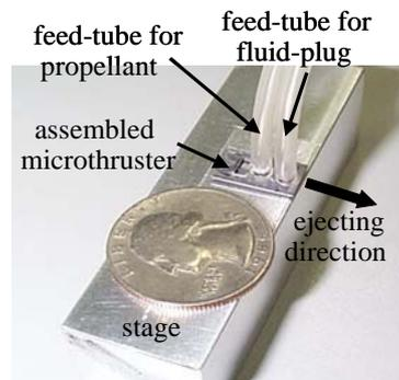
Figure 6. The fabricated microthruster, attached on the stage.
