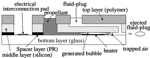
Figure 2. Cross-sectional view of the microthruster.
