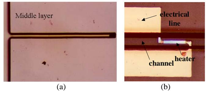
Figure 5. Photograph of the fabricated microchannel (b), showing the enlarged view of the region B in Fig.3(b), and heater (a), showing the top view of the region C in Fig.3(c).
