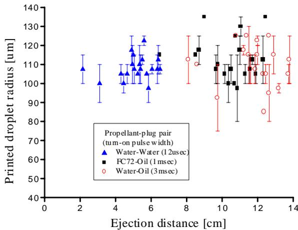
Figure 8. Measured ejection distances and printed radii of 20 ejected droplets, when 7Hz square wave voltage of 13V is supplied to the microheater of  $420\pm 0.5\Omega$ .
