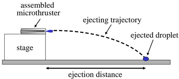
Figure 7. Illustration of the impulse measurement test.
