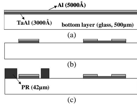
Figure 4. Fabrication process for the bottom layer of microthruster, showing the cross-section along A-A' in Fig. 3: (a) Al/TaAl sputtering; (b) Al/TaAl patterning; (c) thick PR molding.
