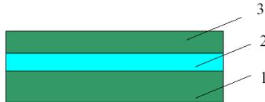
(b) A second layer (3) has been deposited on top of stop layer (2). The second layer (3) should have low thermal conductivity such as SiO<sub>2</sub>.
