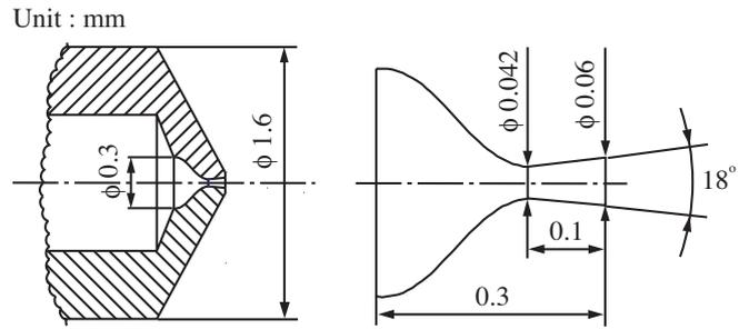
Figure 2. Schematic drawing of the micro nozzle.
