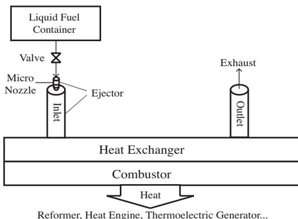
Figure 1. Configuration of micro heat generation system.
