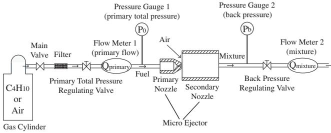
Figure 6. Experiment setup for micro ejector.
