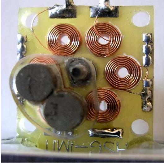
Figure 5: Prototype of an inductive non-resonant vibration transducer
