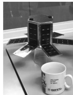
Figure 7: PalmSat model with deployed solar panels, compared with coffee mug.
