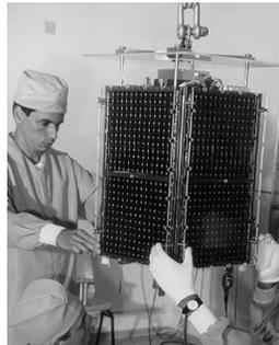
Figure 2: Small spacecraft with fixed arrays mounted on body(PoSat)
