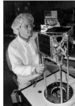
Figure 3: SNAP during testing, showing 3 of the 4 solar panels (base area occupied by launcher separation system)
