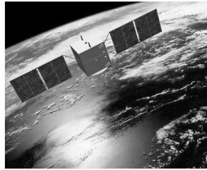
Figure 1: Large spacecraft with deployable, steerable solar arrays
