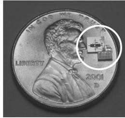
Figure 10: 'Golem dust' solar powered mote with accelerometer, light sensor and RF transceiver (UC Berkeley, BSAC)
