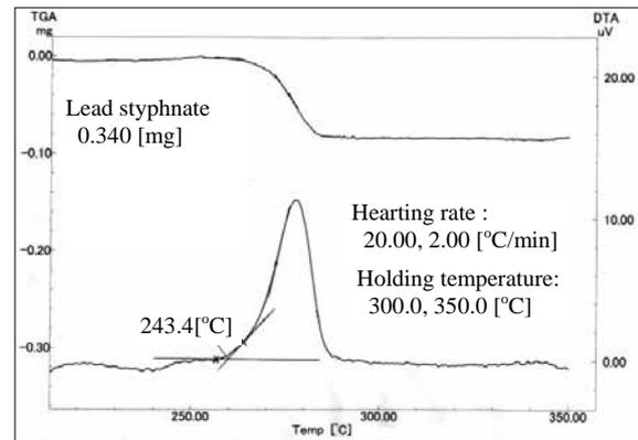
Fig. 4 DTA/TGA curves of lead styphnate
