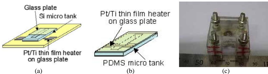
Fig. 1 Test chips (a), (b) and picture of jig (c)
