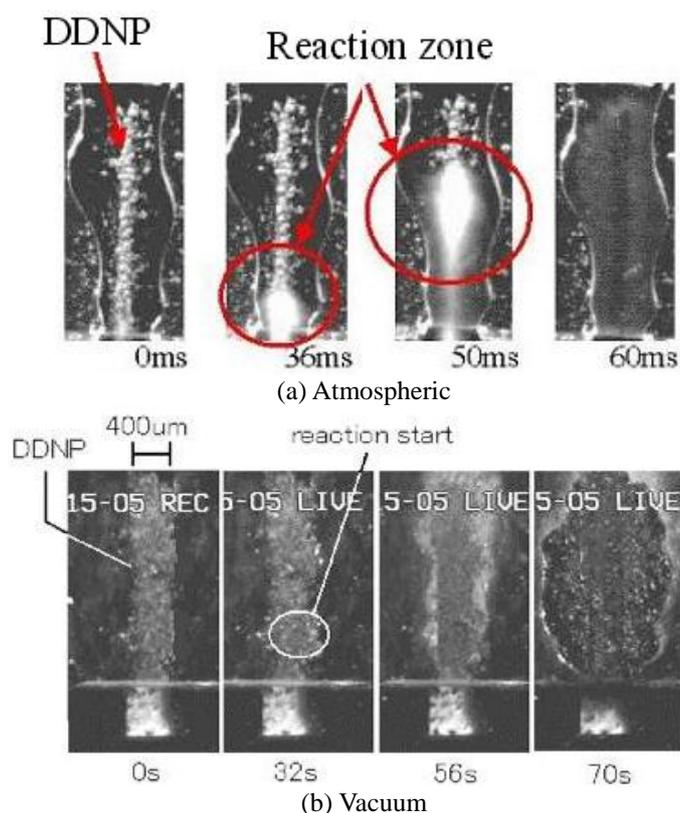
Fig. 2 Snapshots of DDPN in open-end tank ignited by 5W heater.
