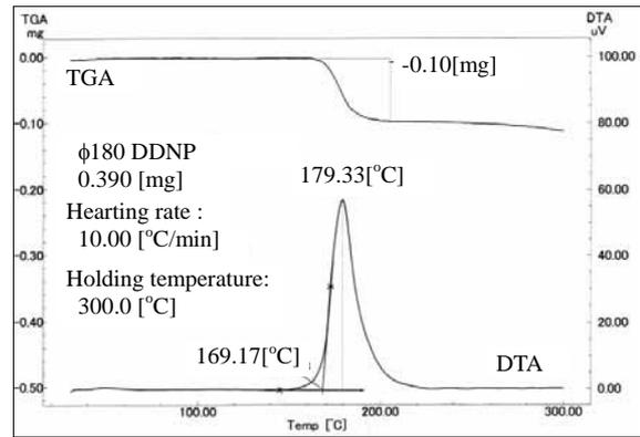
Fig. 3 DTA/TGA curves of DDNP
