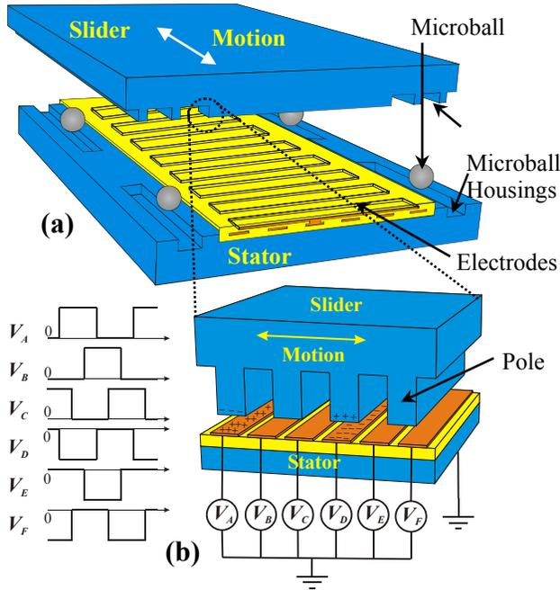
**Figure 1.** (a) Schematic 3D view of the six-phase, bottom-drive, linear, variable-capacitance micromotor, and (b) principle of operation and square-wave excitation.
