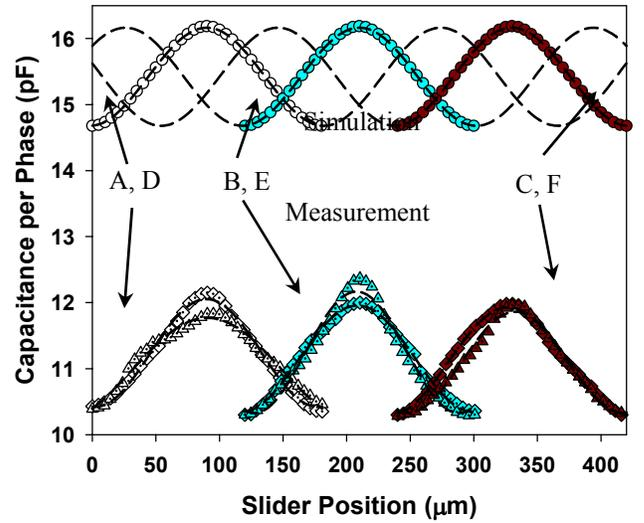
**Figure 4.** Simulated and measured capacitance of all B-LVCM six phases for device D2. The data is fit to sine-squared functions.
