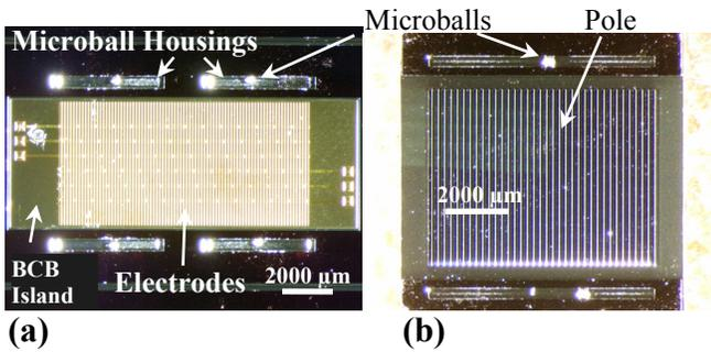
**Figure 3.** Optical micrograph of (a) a fabricated stator and (b) a DRIE-fabricated slider.
