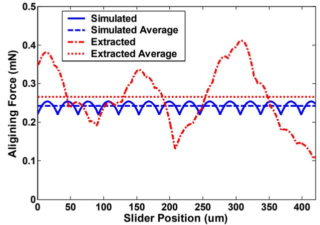
**Figure 5.** Simulated and extracted total aligning force and their average values. The force is calculated from curve fits to simulated and measured capacitance data of Figure 4.
