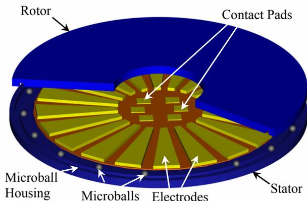
**Figure 6.** Schematic 3D view of the six-phase, bottom-drive, rotary, variable-capacitance micromachine.
