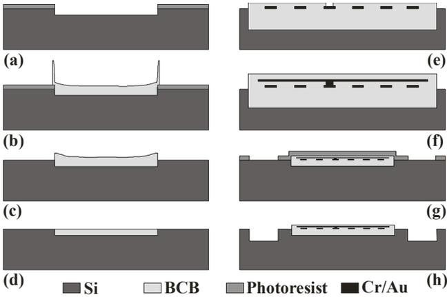
**Fig. 2.** Major process steps for fabrication of the B-LVCM stator: (a) etch Si pit with DRIE, (b) spin-cast and pattern photo-BCB, (c) lift off BCB ridges, (d) planarize EBiS island with CMP, (e) fabricate Cr/Au interconnects and pattern photo-BCB to open vias, (f) fabricate Cr/Au electrodes and pattern photo-BCB passivation layer, (g) and (h) etch trenches with DRIE.
