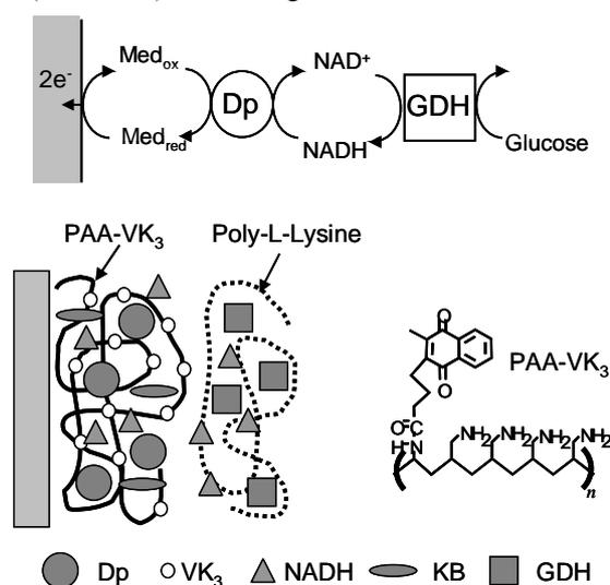
**Figure 2** Schematic illustration showing structure of enzyme anode with expected reaction
