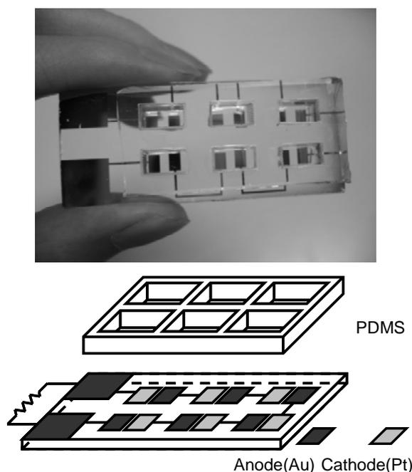
**Figure 5** Biofuel cells stacked on a chip.
