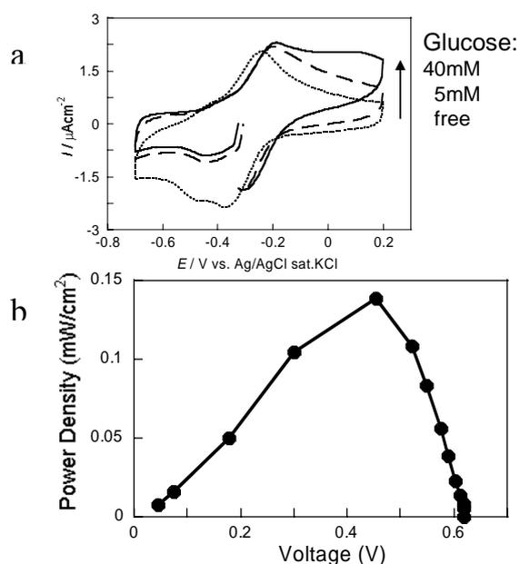
**Figure 3** Cyclic voltammograms of the enzyme anode, and cell performance in 5 mM glucose buffer solution at 37 °C.
