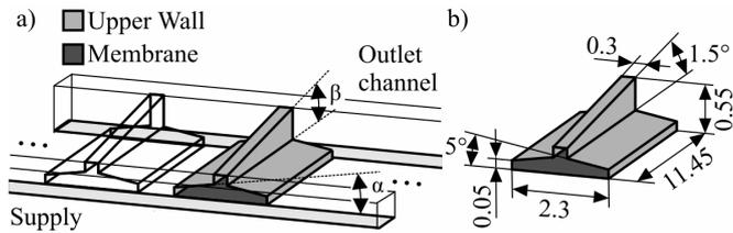
Figure 1. a) Draft of one side of the flowfield indicating the supply and outlet channel as well as the T-shaped parallel channels with their inclination angles  $\alpha$  and  $\beta$ . b) Sketch of the channel dimensions of the test samples in mm (not to scale)
