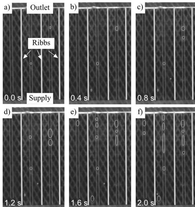
Figure 5. Picture sequence of gas bubbles developing with a 2 M methanol solution inside one test sample.
