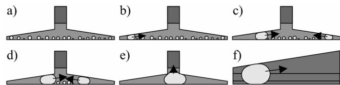
Figure 2. Schematic view of the working principle for the gas bubble movement inside a T-shaped channel.
