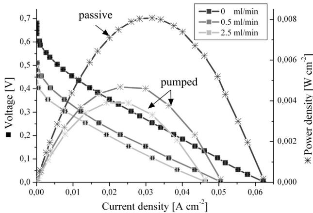
Figure 6. Short time measurements with a 4 M methanol solution at two pumped flow rates and a passive system setup.
