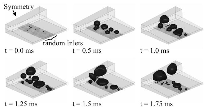
Figure 3. Simulation sequence with distributed bubble sources and bubble removal due to capillary forces. The symmetry of the channel is used to simplify the model.
