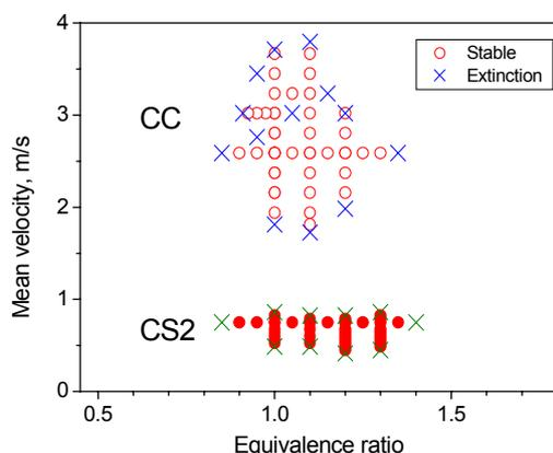
Fig. 6 Flame stabilization of coin-size combustors (CC and CS2)
