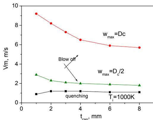
Fig. 5 The effect of the cap thickness of the combustor on flame stabilization for coin-size combustors
