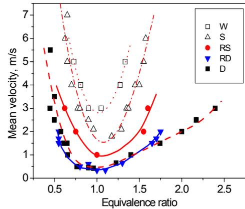
Fig. 2. Flame stabilization conditions of various combustors
