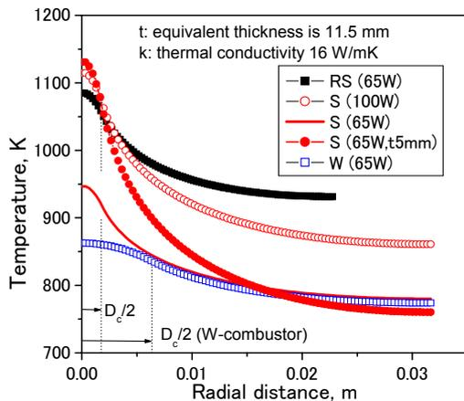
Fig. 4 Temperature distribution and flame stabilization estimated using a simple one-dimensional model
