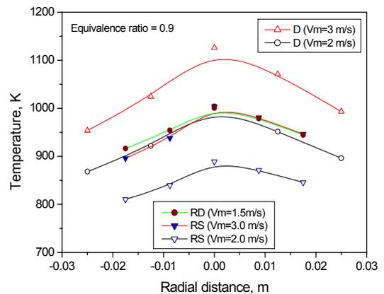
Fig. 3. Similarity in temperature distribution between different scale combustors
