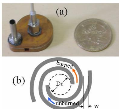
Fig. 1. (a) 500-Yen size combustor (CC-combustor in Table 1), (b) Configuration at the center.
