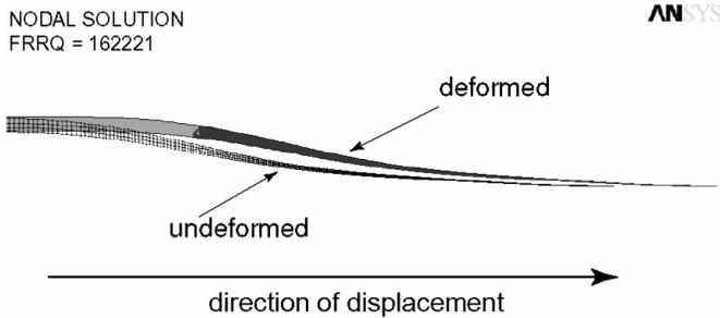
**Figure 3** – The compression and expansion in the neck of the actuator responsible for droplet ejection [5], as simulated in ANSYS, with an axisymmetric model of the actuator.
