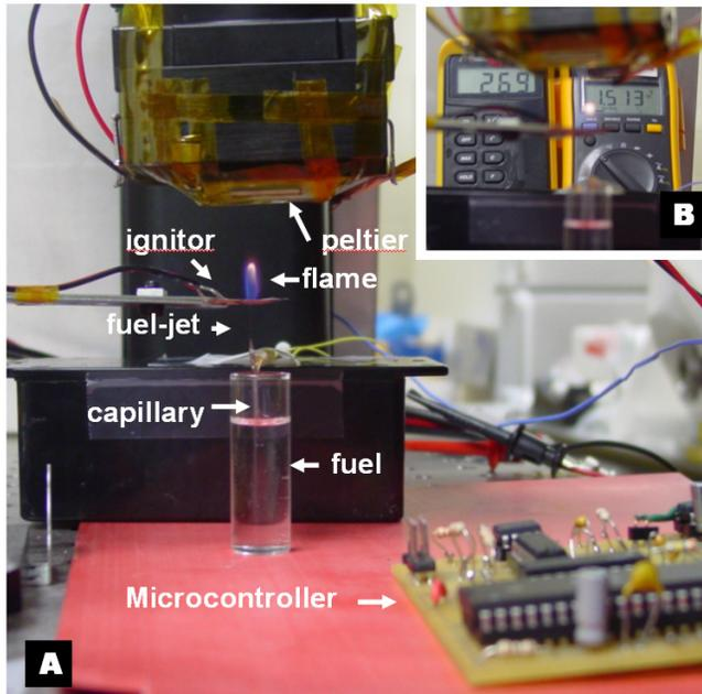
**Figure 4** – Description of the experimental setup for power generation (A) with open circuit voltage reading of 1.5V at 270°C (B).
