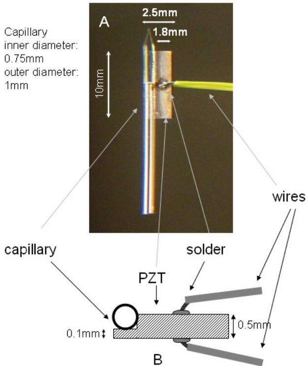
**Figure 1** – Picture of the composite actuator (A) with the schematic drawing of the side view (B).
