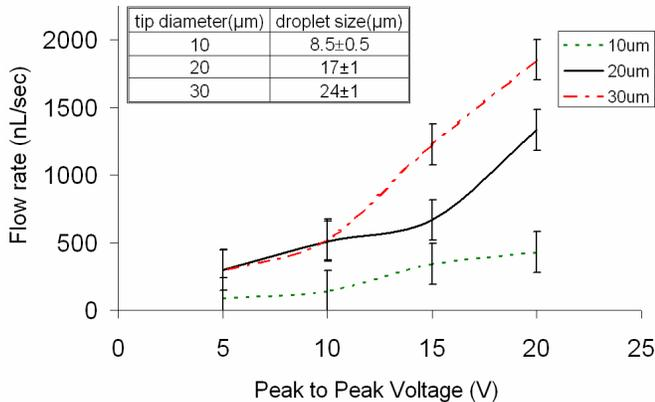
**Figure 6** – Flow rate with driving voltage for different tip diameters.
