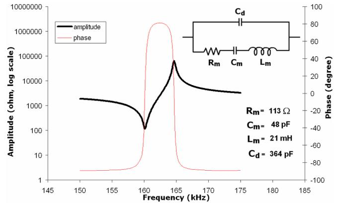
**Figure 2b** – The input impedance amplitude and phase of the overall actuator  $Q:420$   $K_{eff}^2:0.057$  and equivalent electrical circuit of a typical PZT/capillary resonator.
