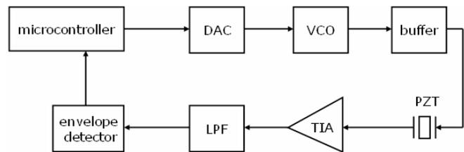
**Figure 5** – Block diagram of the microcontroller based lock-in circuit ( $\mu$ -controller: Atmel-Mega32 Buffer: MCP601).
