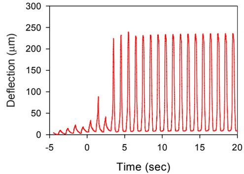
**Figure 4** - Dynamic deflection of the top expander membrane of the engine at 1 Hz.
