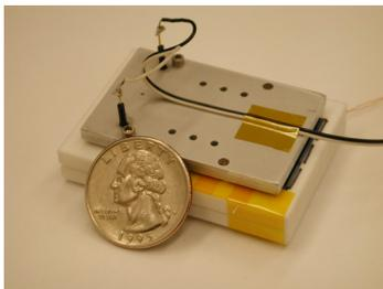
**Figure 3** - Completed dynamic micro heat engine.
