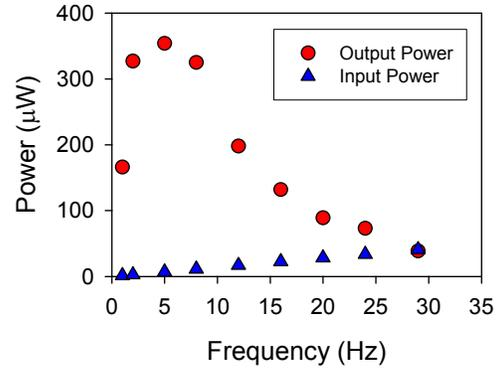
**Figure 8** - Mechanical power out of the micro engine and mechanical power into the thermal switch as functions of micro engine cycle speed.
