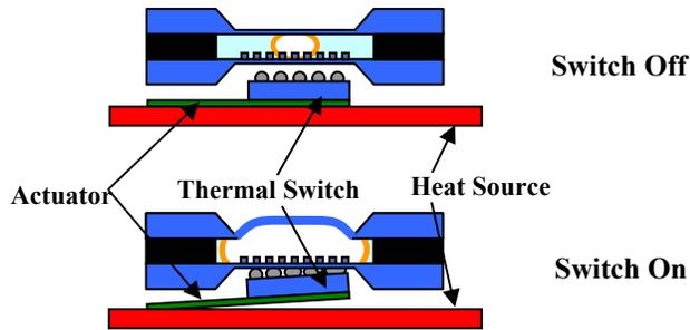
**Figure 2** - Schematic of engine with cantilever switch.
