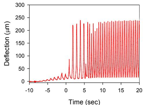
**Figure 5** - Dynamic deflection of the top expander membrane of the engine at 2 Hz.
