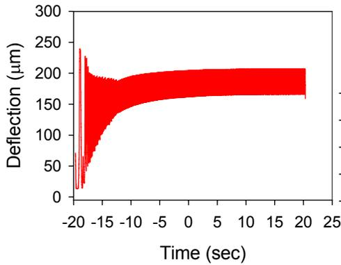
**Figure 6** - Dynamic deflection of the top expander membrane of the engine at 16 Hz.
