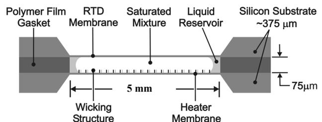
Figure 1 - Cross section of micro heat engine.
