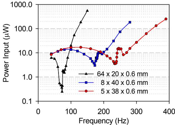
**Figure 10** - Thermal switch power input versus frequency for three cantilever switches with 40  $\mu\text{m}$  deflection.
