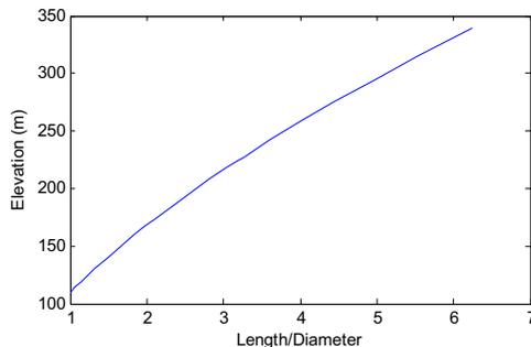
**Figure 1** – Theoretical elevation limit from various  $L/D$  ratios using 130mg of AP/HTPB propellant, assuming  $I_{sp} = 120s$ ,  $C_d = 0.4$ ,  $r = 10mm/s$ ,  $MR=2$ .
