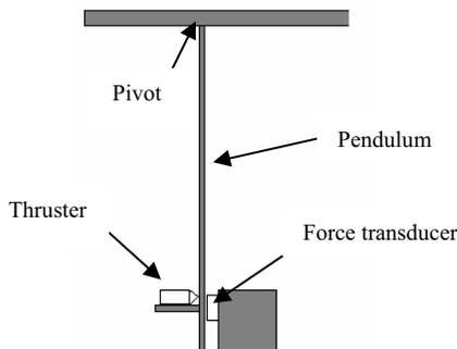
**Figure 5** - Schematic of thrust measuring apparatus.
