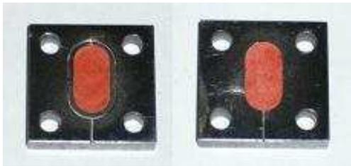
**Figure 4** – Circulating rectangular nozzle and baseline short nozzle before testing.
