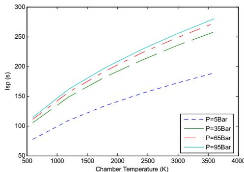
Figure 3 – Isentropic  $I_{sp}$  for various temperatures and pressures.
