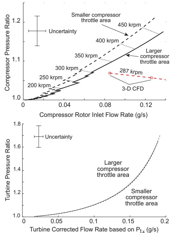
**Figure 5 –** Compressor map (top) and turbine map (bottom).
