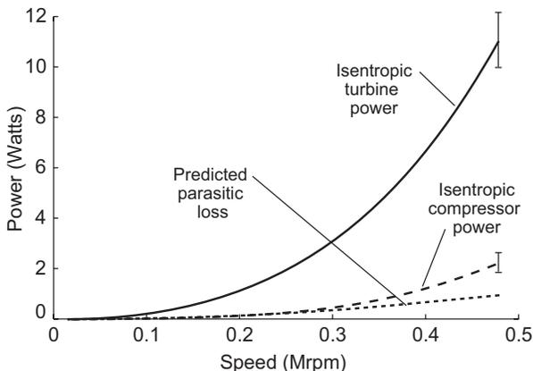
Figure 6 – Isentropic power to turbine and from compressor, and predicted parasitic loss.
