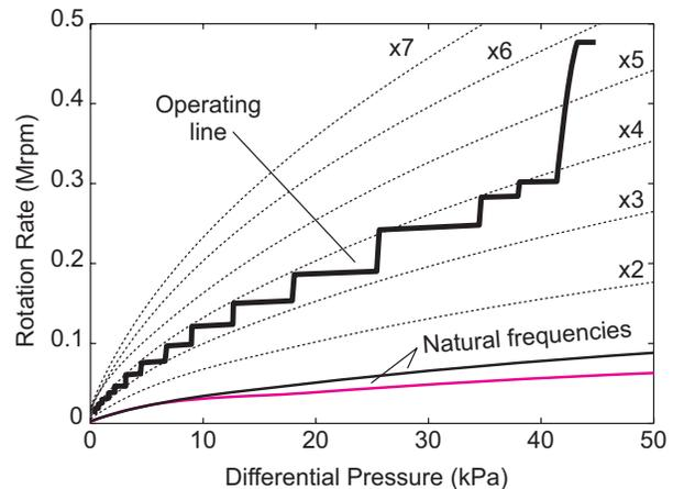
**Figure 3** – Rotordynamic acceleration map for test 1. Operating schedule chosen to initially stay between the 3<sup>rd</sup> and 4<sup>th</sup> multiple of the larger natural frequency.
