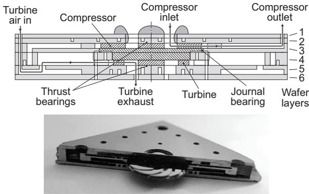
**Figure 2** - Turbocharger cross-section. The hatched region in the top figure denotes the rotor.
