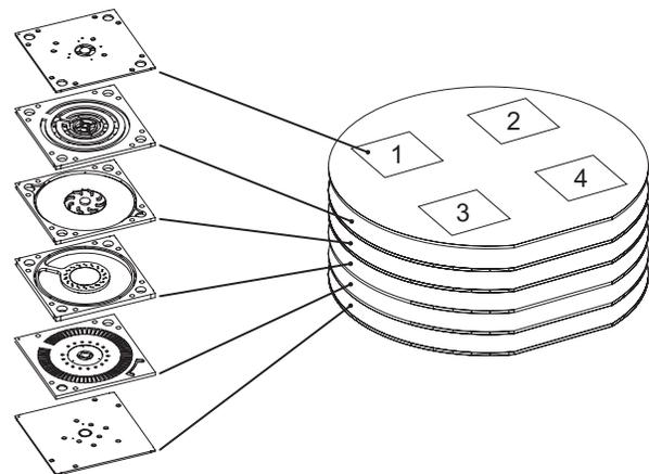
**Figure 1** - The turbocharger is formed by fusion bonding six wafers to form four separate devices in the corners. The large die separation improves etch uniformity during the highly loaded blade etches.
