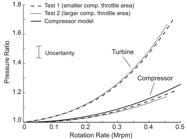
**Figure 4 –** Pressure ratios measured across the compressor and turbine.
