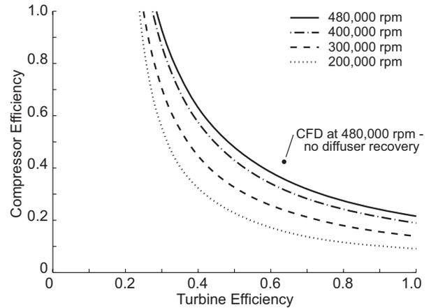
Figure 7 – Turbine/compressor efficiency relations based on measured spool performance and predicted parasitic losses.
