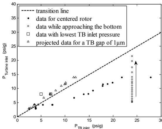
**Figure 5** - Turbine versus thrust bearing inlet pressures. By reducing the thrust bearing gap, it is shown analytically and experimentally that the bearings can be operated with a single feed at the turbine inlet pressure.
