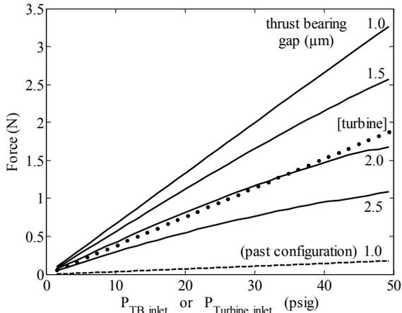
**Figure 2** - Relative force produced on the bottom of the rotor for the new configuration (ports 4, 5 and 6 closed) compared to the past configuration (dashed lines, ports 4, 5 and 6 open). The dotted line is the downward turbine force as a function of its inlet pressure. Keeping the thrust bearing gap under 2 $\mu$ m leads to a lower inlet pressure for the thrust bearing compared to the turbine.
