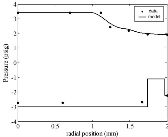
**Figure 4** - Validation of the start-up procedure with low thrust bearing pressure (3.8psig). The rotor was stable and running at 24 500 RPM. The thrust gap for the analytical simulation was 2  $\mu\text{m}$ .
