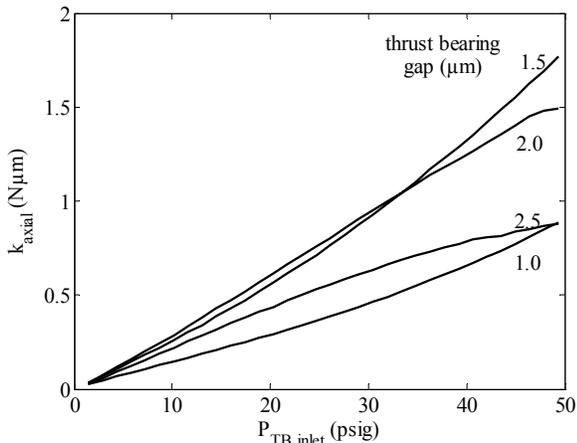
**Figure 3** - Axial stiffness produced by the pressure field under the rotor for the new configuration proposed (ports 4, 5 and 6 closed).
