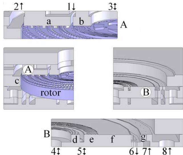
**Figure 1** - Components around the rotor ; turbine (a), top seal (b), journal bearing (c), pump (d), bottom seal (e), axial balance plenum (f) and peripheral thrust bearing (g). Numbers are referring to different ports where flows can come in or out. On B view, the rotor and the two top layers are removed.
