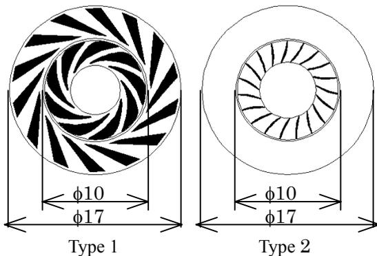
Figure 6 Designed blade shapes for rotation test using the air turbine.
