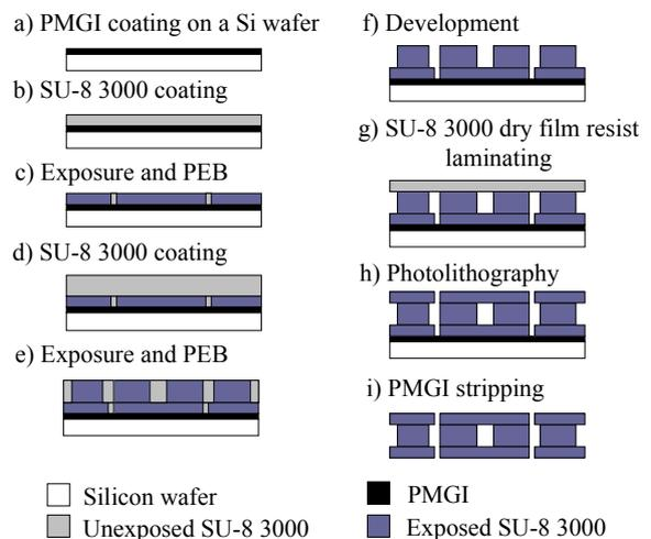
Figure 1 Fabrication process of SU-8 impellers.
