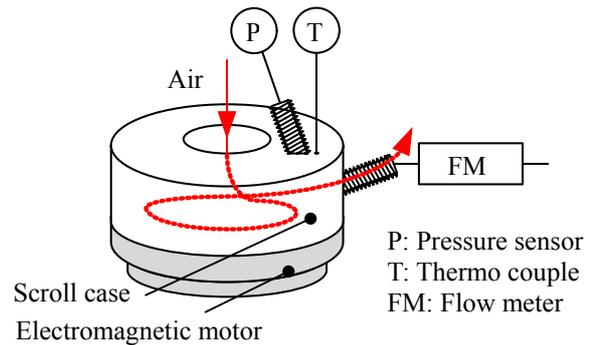
Figure 4 Test setup using the electromagnetic motor.
