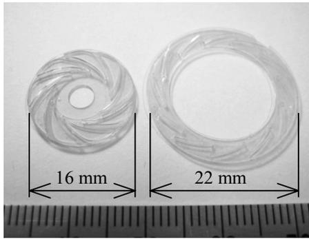
Figure 2 Fabricated impeller and diffuser.
