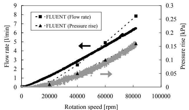
Figure 5 Measured and simulated performance of the 16 mm diameter impeller.
