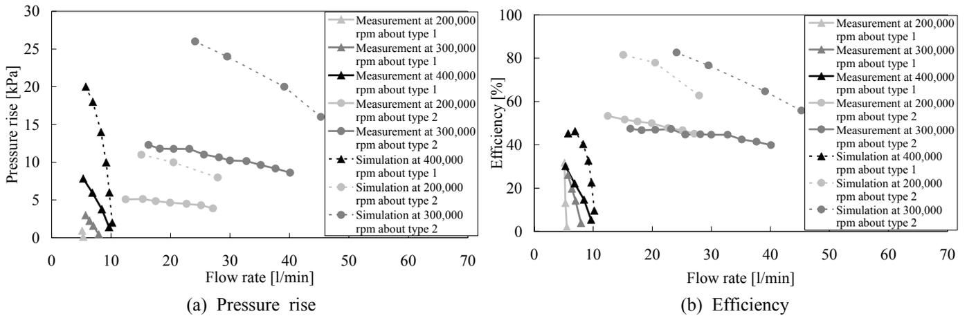
Figure 9 Measured and simulated compressor performance.
