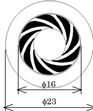
Figure 3 Designed blade shape for rotation test using the electromagnetic motor.
