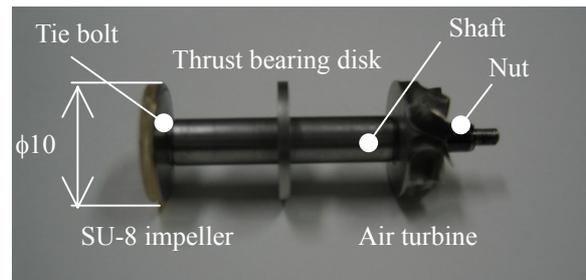
Figure 8 Rotor with the SU-8 microimpeller.
