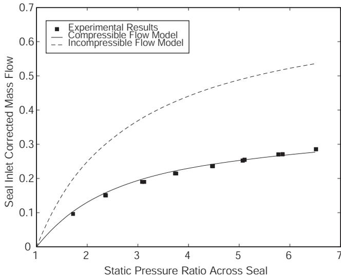
**Figure 4** – Experimental measurements and model predictions of seal inlet corrected mass flow for various labyrinth seal static pressure ratios in a MEMS-turbopump.
