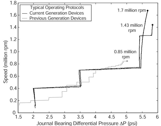
**Figure 5** – Comparison of typical operating protocols for previous and current generation MEMS air-turbines. Maximum rotor speed for current generation devices is 1.7 million rpm.
