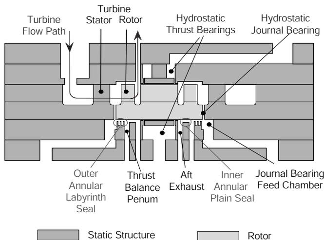
**Figure 1** – Cross sectional view of the gas-bearing supported MEMS-air turbine (not to scale).
