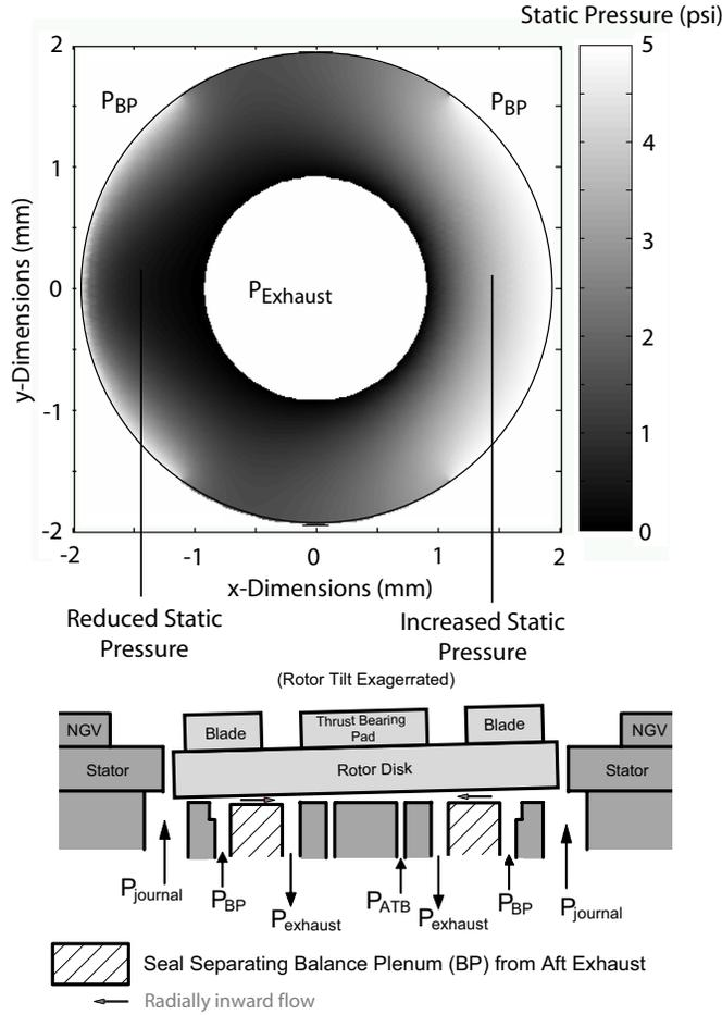
**Figure 3** – Annular seal static pressure distribution for a rotor tilting angle of  $-0.0006$  radians equivalent to a rotor tip deflection of  $1.3 \mu\text{m}$ .
