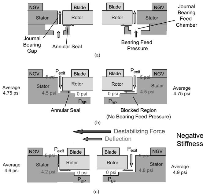
**Figure 2** – (a) Journal bearing flow in unblocked region. (b) and (c) Mechanism for negative (destabilizing) radial stiffness due to coupling of reverse flow through journal bearing land and annular seal in blocked region.
