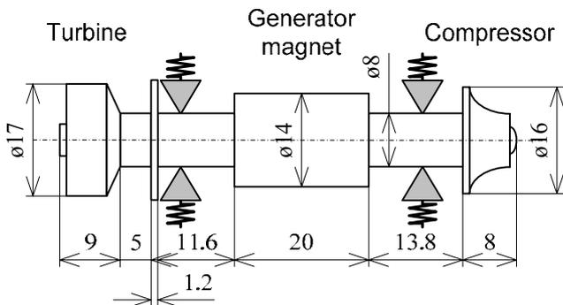
Figure 2 Structure of the designed rotor.
