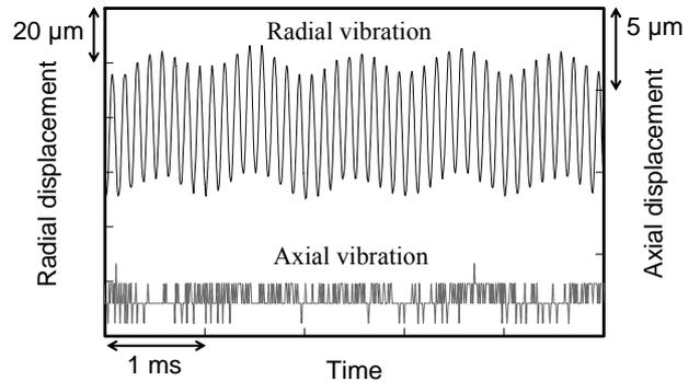
Figure 8 Waveform of the rotor vibration at 480000 rpm.
