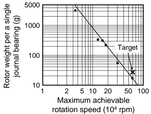
Figure 4 Empirical trend between the maximum achievable rotation speed and the rotor weight per a single journal bearing (reproduced from [4]).
