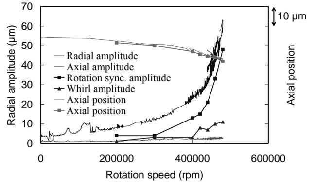
Figure 7 Radial amplitude and axial position of the rotor.
