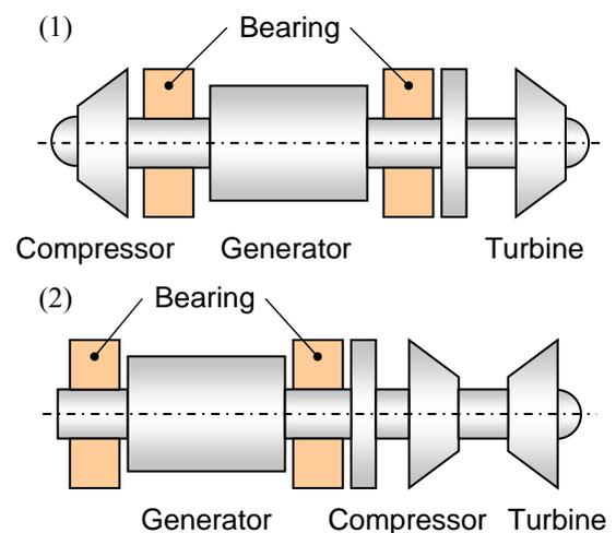
Figure 1 Typical layout of rotors.
