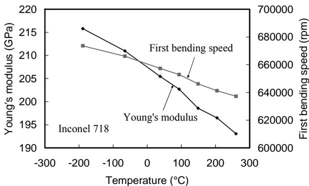
Figure 3 Calculated first bending resonant speed vs. temperature.
