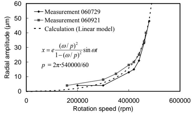
Figure 9 Amplitude of the rotation-synchronous vibration and fitting by a linear spring-mass model.
