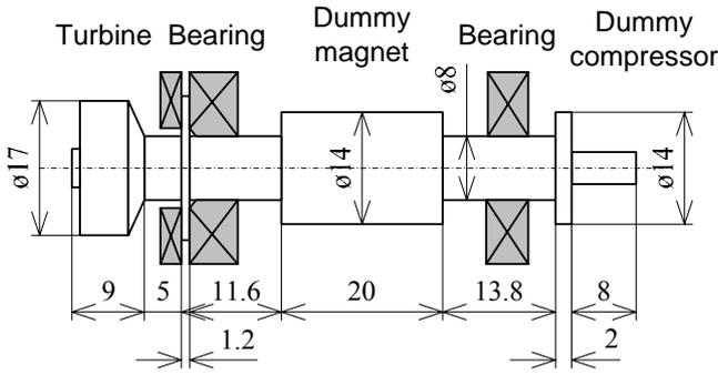
Figure 6 Layout of the rotor and bearings.
