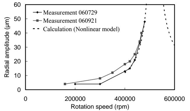
Figure 10 Amplitude of the rotation-synchronous vibration and fitting by a nonlinear spring-mass model.
