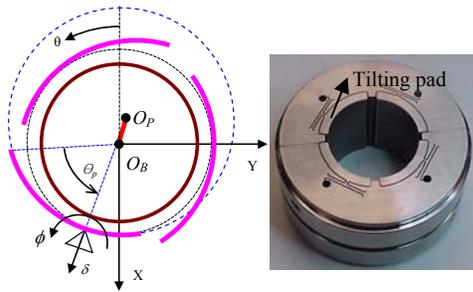
**Figure 2** – Principle of tilting pad gas bearing and EDM machined 4 pads flexure pivot tilting pad gas bearing
