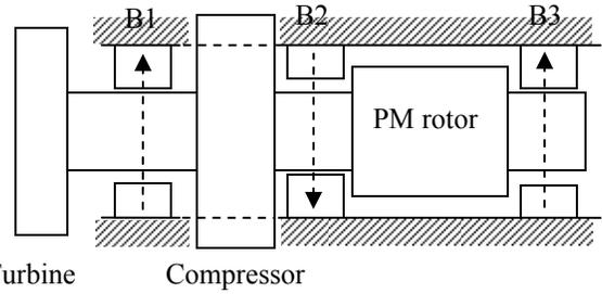
Figure 8 – Arrangement of loaded foil bearings, arrows indicate the direction of loadings
