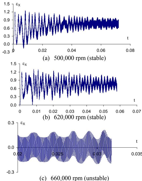
Figure 7- Selected time traces of  $\epsilon_x$  for foil bearing with external load of 0.5N
