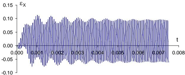
Figure 6 – Simulated time trace of  $\epsilon_x$  for tilting pad gas bearing at 800,000 rpm
