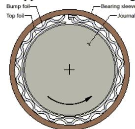
Figure 1 - Schematics of foil gas bearing [8]
