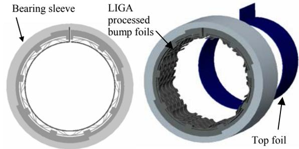
(a) Top view of assembled foil bearing (b) Assembly scheme
