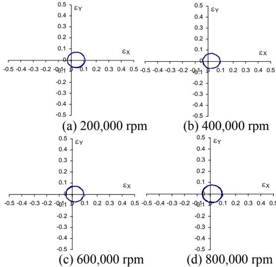
Figure 5 – Selected orbits for tilting pad gas bearings
