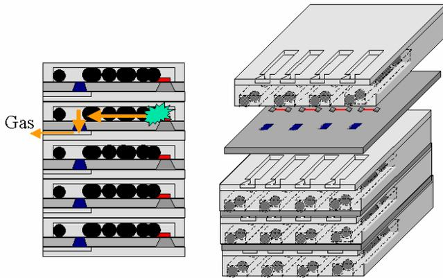
**Figure 4** – 3D view of micro rocket array. The combustion starts at the igniter and propagates producing high-temperature gas which bursts the upstream membrane. The gas goes through the bulk-etched silicon substrate and PDMS nozzle and then thrust is yielded.
