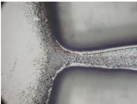
**Figure 5** – Microscopic image of the nozzle after firing test. The throat is not clogged and also other part of PDMS structure is not damaged.
