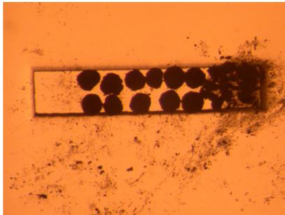
(a) DDNP balls in PDMS tank before ignition
