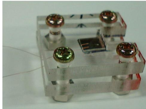
**Figure 6** – Setup device for thrust measurement. The micro rocket is sandwiched by two acrylic places, which are pressed by screws to prevent burned gas leakage.
