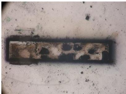
(c) PDMS tank after ignition of 1.0W power
