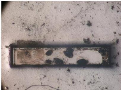
(b) PDMS tank after ignition of 0.5W power
