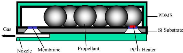
**Figure 1** – Schematic of the proposed micro rocket using DDNP propellant and PDMS tank and nozzle. The height of tank is designed slightly shorter than the diameter of DDNP balls.
