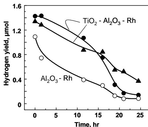
**Figure 4** Hydrogen yield from propane partial oxidation over (a) Al<sub>2</sub>O<sub>3</sub>, (b) TiO<sub>2</sub> – Al<sub>2</sub>O<sub>3</sub> (TiO<sub>2</sub> wt.% 54), and (c) TiO<sub>2</sub> – Al<sub>2</sub>O<sub>3</sub> (TiO<sub>2</sub> wt.% 40)
