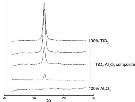
**Figure 1** Slow – scan XRPD pattern of the mixed oxide with different compositions From bottom to top: Ti(0), Ti(0.25), Ti(0.43), Ti(0.64), and Ti(1). The only peak observed in the figure corresponds to anatase phase of  $\text{TiO}_2$ .
