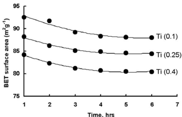
**Figure 2** This figure shows the surface area of the mixed oxide after calcination at 900°C. The surface area of the oxide is stable following several heat – cool cycles.
