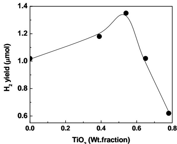
**Figure 3** This figure shows the Hydrogen yield from propane partial oxidation over TiO<sub>2</sub>-Al<sub>2</sub>O<sub>3</sub> of different weight ratios. Operating conditions: Rh – 3.5±0.02wt %, flowrate 305 sccm.
