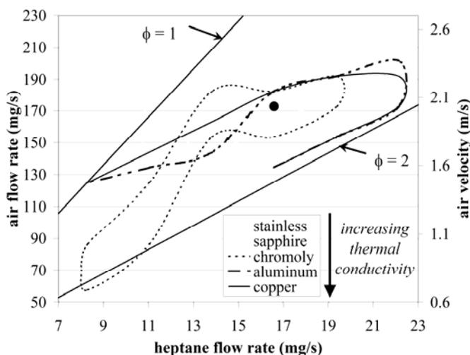
**Figure 5.** Fuel flow rates and air flow rate operating regimes for combustors constructed of materials with various thermal conductivity.
