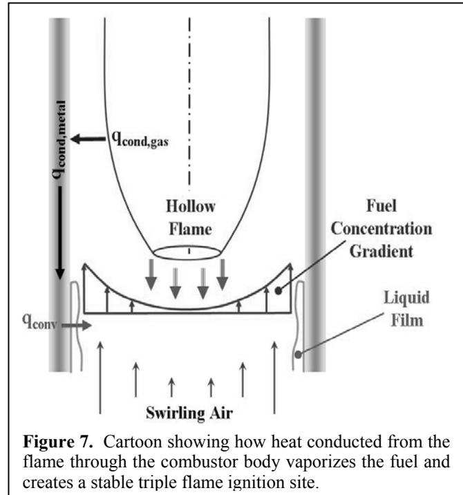
**Figure 7.** Cartoon showing how heat conducted from the flame through the combustor body vaporizes the fuel and creates a stable triple flame ignition site.
