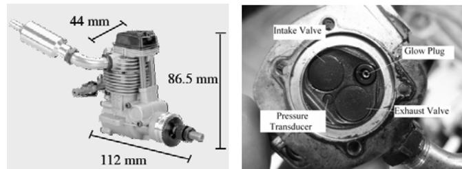
**Figure 1.** Miniature 4-stroke model airplane engine (left) and the engine head from the engine showing the location of the pressure transducer
