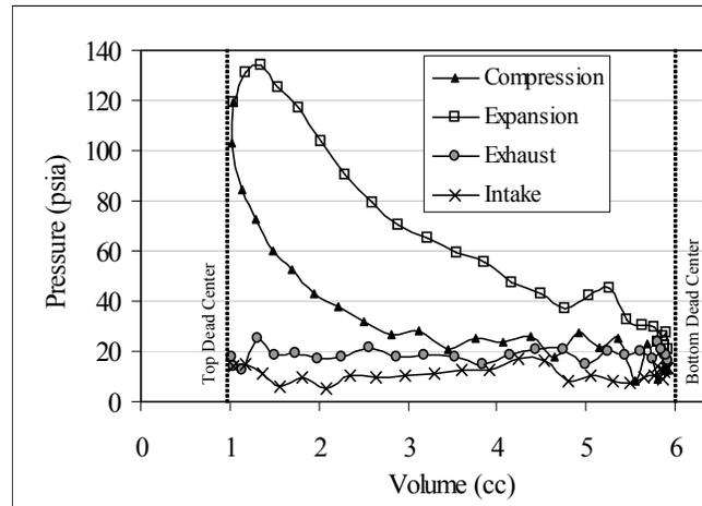
**Figure 3.** Indicator diagram for a single 4-stroke cycle of the miniature piston engine.
