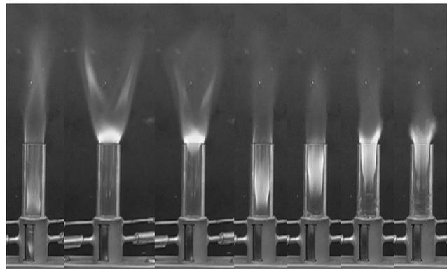
**Figure 4.** Images of the film combustor operating on heptane. Air flow rate increases left to right.
