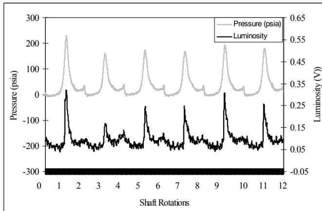
**Figure 2.** Pressure (upper trace) and luminosity (lower trace) inside the miniature piston engine cylinder during operation.
