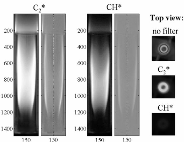
**Figure 6.** Chemiluminescence images of the film combustor. The image to the left is the normal camera image and the one to the right is the Abel transformed version. The three round images are top views confirming the hollow core of the film flame.
