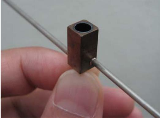
Figure 8 – Photo of micro cyclone combustor (Model 2).
