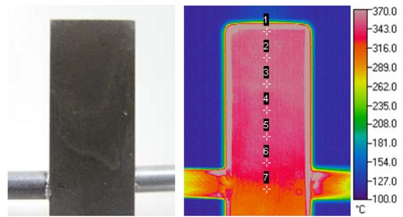
**Figure 6** - Real and thermal images of the micro cyclone combustor wall without the outer housing.
