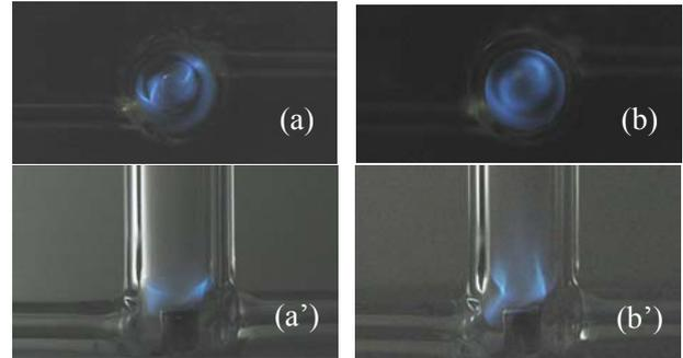
**Figure 3** - Photos of the flame shape inside the micro cyclone combustor; Upper : top view, Lower : side view; (a) and (a') :  $Q_{\text{fuel}} = 52.3 \text{ sccm}$ ,  $\Phi=1.0$ , (b) and (b') :  $Q_{\text{fuel}} = 52.3 \text{ sccm}$ ,  $\Phi=0.8$ .
