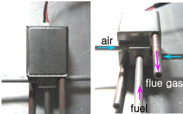
**Figure 5** - Photos of the micro cyclone combustor integrated with the outer housing.
