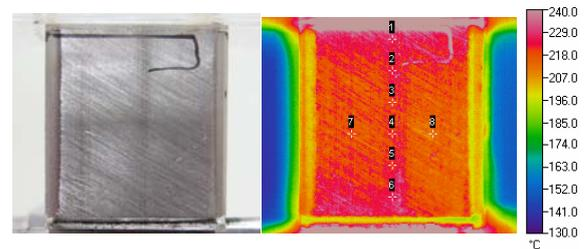
**Figure 7** - Real and thermal images of the outer housing wall of the micro cyclone combustor.
