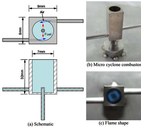
**Figure 2** - Schematic and photo of the micro cyclone combustor (Model 1); (c) :  $Q_{\text{fuel}} = 52.3 \text{ sccm}$ ,  $\Phi=1.0$ .
