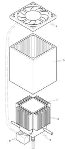
**Figure 1** - Schematic of the unit thermoelectric power generator integrated with a combustor; 1 : thermoelectric module, 2 : combustor, 3 : cooling fins, 4 : cooling fan, 5 : outer housing, 6 : storage capacitor.
