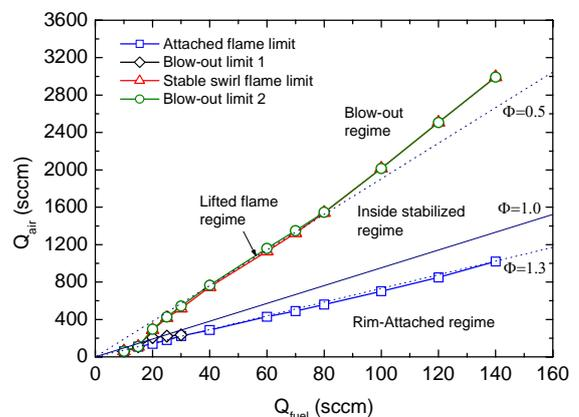
**Figure 4** - Combustion stability diagram of the micro cyclone combustor.
