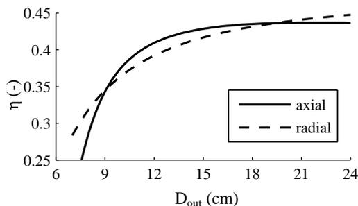
**Figure 5** – Cycle efficiency vs. outer diameter for an axial design (—) and a radial design (---)
