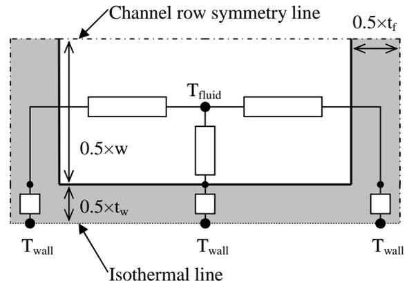
**Figure 2** – Unit cell with parallel thermal resistances connected to an isothermal plane between hot and cold channels.
