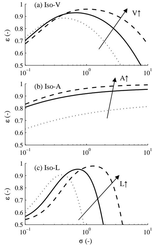
**Figure 3** – Iso-V, Iso-A and Iso-L curves for baseline dimensions (—), half baseline dimensions (···) and double baseline dimensions (---) for  $\Delta p_h = 8$  kPa and  $\Delta p_c = 12$  kPa
