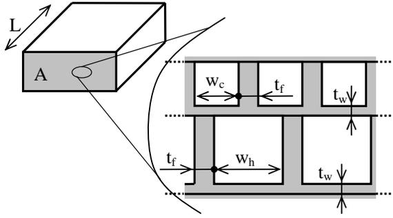
**Figure 1** – Schematic of the micro channel heat exchanger
