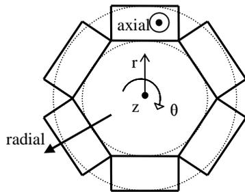
**Figure 4** – Constant z section of the annular heat exchanger with axial or radial flow directions
