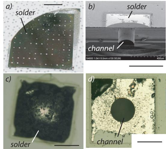
FIG. 4: a) Front side of a quarter of 3 inch wafer after fabrication. The alloy parts are clearly seen. Bar length is  $1\ \text{cm}$ ; b) SEM micrograph of the cross section of one device. Bar length is  $400\ \mu\text{m}$ ; c) Optical micrograph of the front side of one device in the closed position. Bar length is  $200\ \mu\text{m}$ ; d) Optical micrograph of the front side of one device after being opened. Bar length is  $200\ \mu\text{m}$ .
