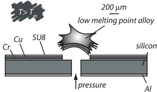
FIG. 2: Scheme showing the cross-section of the device while opening;  $T_m$  is the melting temperature of the low melting point alloy;  $T$  is the ambient temperature.
