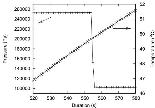
FIG. 5: Temperature sensitivity of the device. Input pressure and temperature as a function of time with increasing temperature. The output pressure is 101 kPa.
