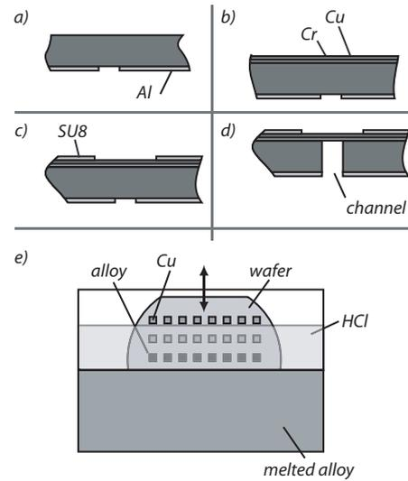
FIG. 3: Illustration of the fabrication process. a) Aluminum deposition and patterning; b) Chromium and copper deposition; c) Su8 deposition and patterning; d) Etching of the channel; e) Low melting point alloy deposition.
