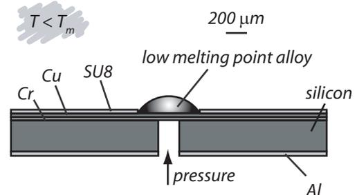
FIG. 1: Scheme showing the cross-section of the device in the closed position;  $T_m$  is the melting temperature of the low melting point alloy;  $T$  is the ambient temperature.
