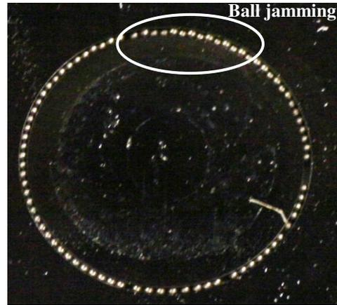
Fig. 8: Optical picture of ball jamming occurring within the ball bearing race.
