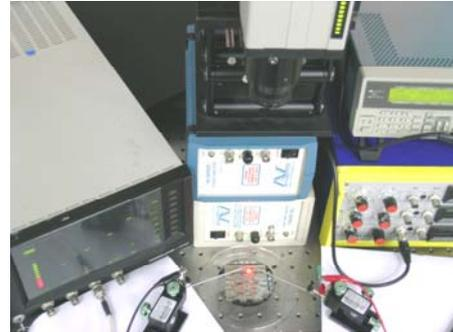
Figure 9 Use laser vibrometer to measure the displacement of devices for characterization of piezoelectric constant.
