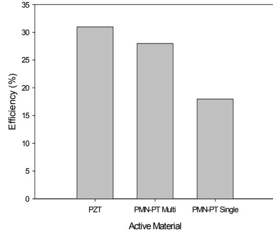
**Fig. 4.** Predicted efficiencies of PZT and PMNPT devices.
