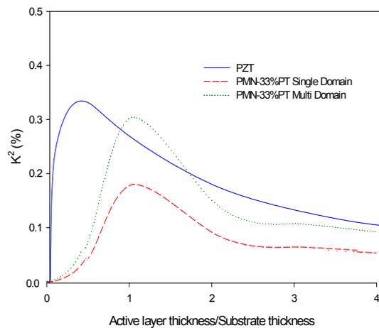
**Fig. 5.** Coupling coefficient as a function of active layer to substrate thickness.
