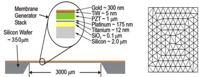
**Fig. 1.** Geometry of device and mesh.
