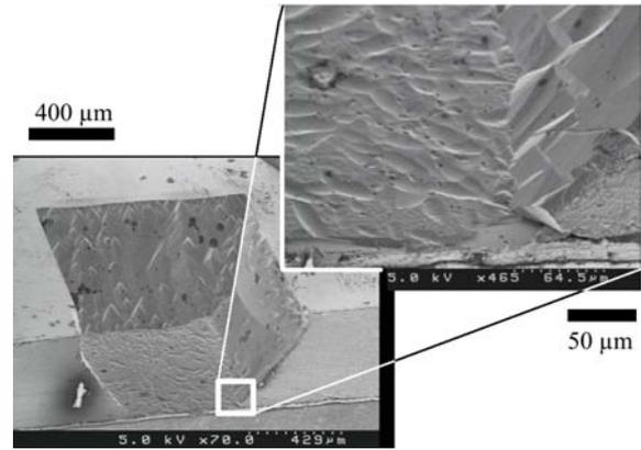
**Figure 13** Diaphragm made in a Z-cut LiNbO<sub>3</sub> wafer for pressure sensing.
