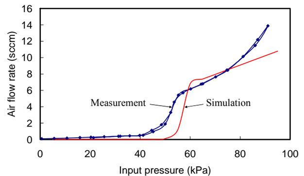
Figure 5 Relationship between input pressure and air flow rate.
