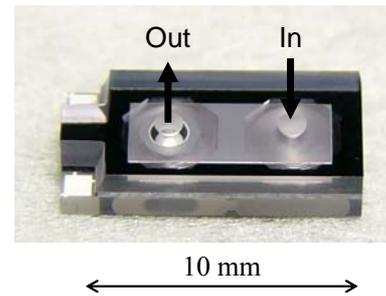
Figure 4 Prototyped microvalve for fuel control in DMFC.
