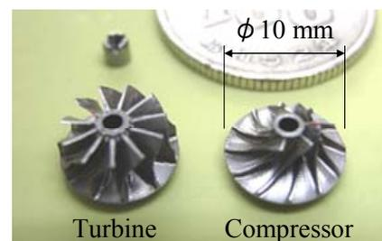
Figure 1 Microimpellers of 10 mm diameter.
