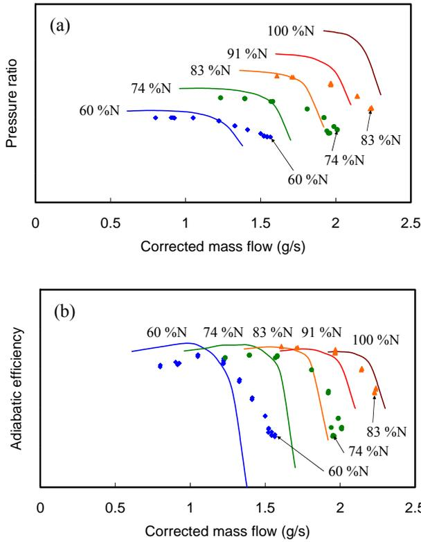
Figure 2 Performance of the micro centrifugal compressor.
