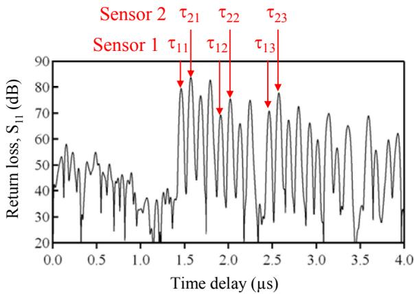
**Figure 11** Returned signals from 4 SAW passive wireless thermometers.
