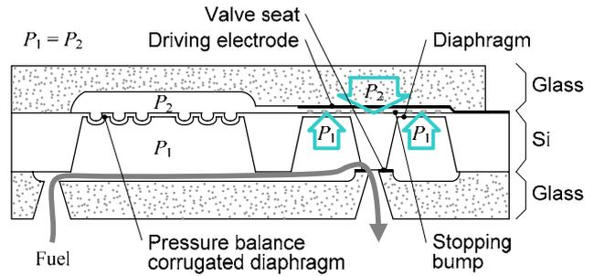
Figure 3 Structure of the electrostatic microvalve with pressure balance mechanism.
