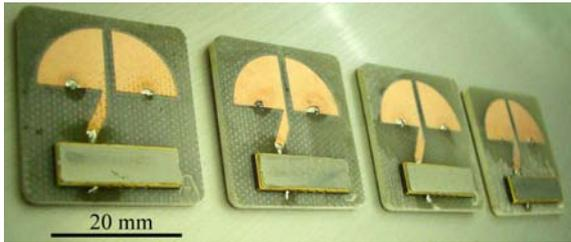
**Figure 10** Prototyped SAW passive wireless thermometers with a patch antenna.
