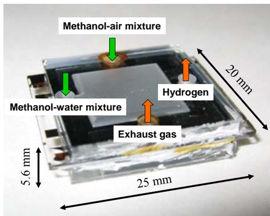
Figure 7 Prototyped micro methanol fuel reformer.
