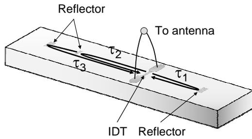
**Figure 9** Working mechanism of SAW passive wireless sensors.
