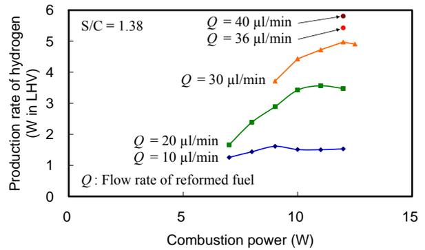
Figure 8 Production rate of hydrogen from the micro methanol reformer.
