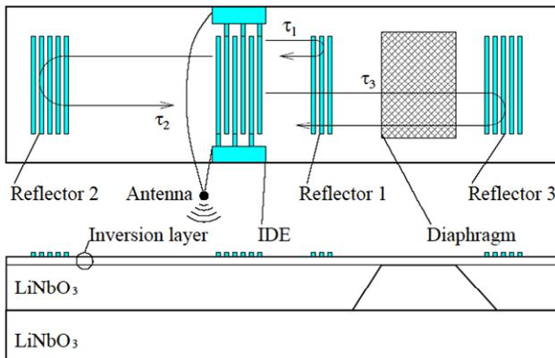
**Figure 12** Structure of a SAW passive wireless pressure sensor.
