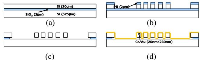
**Figure 6** – Fabrication process for the cross section along A-A' in Fig.4.
