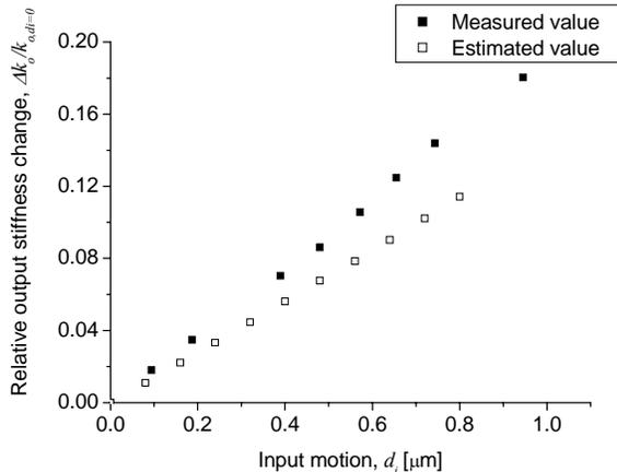
Figure 8 – Estimated and measured relative stiffness change of the variable stiffness spring for varying input motion.
