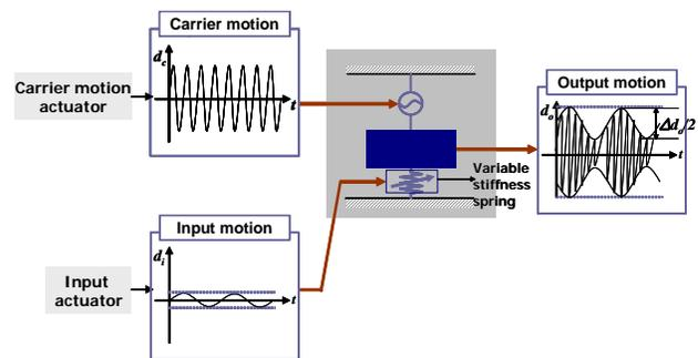
**Figure 1** – Simplified model of the micromechanical energy amplifier
