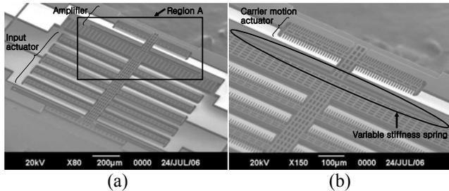
Figure 7 – SEM photographs of the micromechanical energy amplifier: (a) overall structure; (b) an enlarged view of the Region A in (a).
