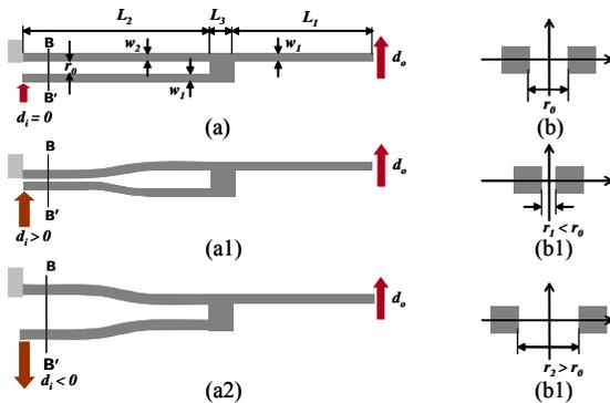
**Figure 5** – Structure and principle of the variable stiffness spring: (a) and (b) illustrate the spring and its cross section of  $BB'$  at the initial input condition of  $d_i=0$ ; (a1) and (b1) showing the spring stiffness reduction at the input condition of  $d_i>0$ ; (a2) and (b2) showing the spring stiffness increase at the input condition of  $d_i<0$ .
