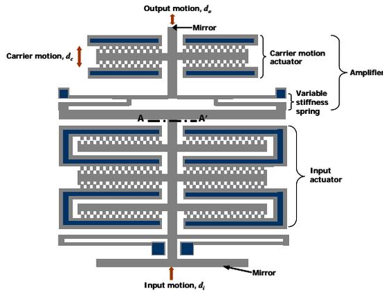
**Figure 4** – Top view of the micromechanical energy amplifier.
