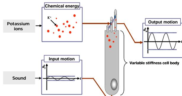
**Figure 2** – Simplified model of the hair-cell energy amplifier.
