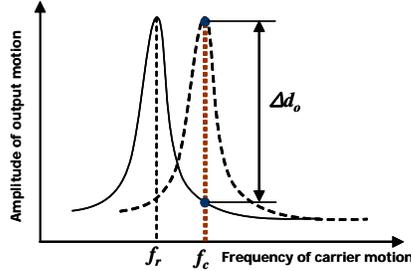
**Figure 3** – Amplified output motion due to the resonant frequency shift from  $f_c$  to  $f_r$ : the resonant frequency shift is caused by the spring stiffness spring (Fig.5) depending on the input motion.
