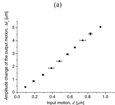
Figure 9 – Estimated and measured relative stiffness change of the variable stiffness spring for varying input motion.
